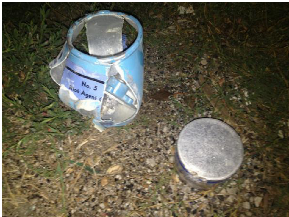
Photo 6 A Smith & Wesson CS grenade, manufactured by the now defunct Smith & Wesson Chemical Co. Note the deformed sides of the munition.
