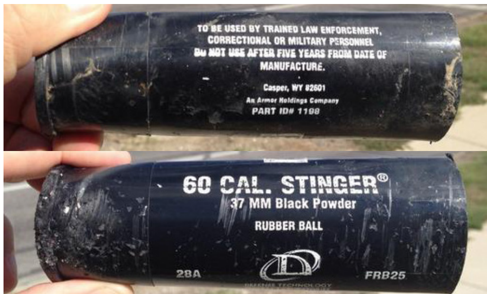
Photo 3 A fired 60 cal. stinger 37mm black powder rubber ball cartridge, manufactured by Defense Technology.
