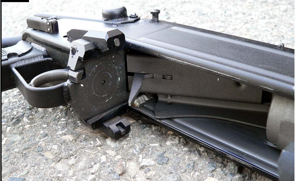
A GM-94 launcher with the barrel in the forward position. Note the stationary breech and barrel locking clamps.
