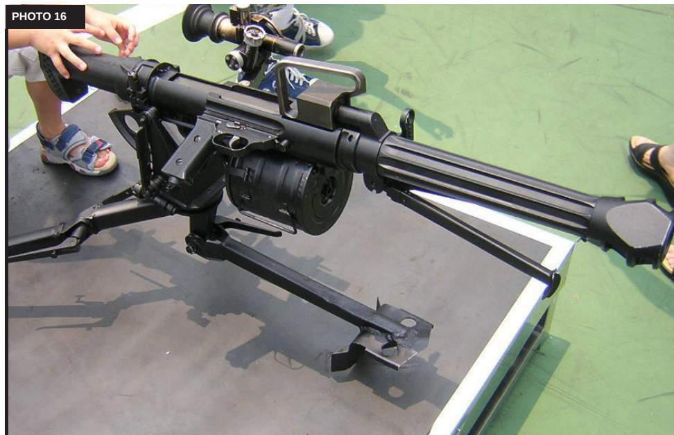
QLZ87 in 'heavy' configuration, with 15-round drum magazine, 3x optical sight, and tripod.
