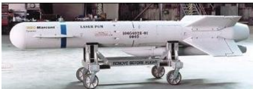
Figure 1.8 – Hakim A1 semi-active laser guided munition. Note GEC-Marconi Dynamics markings.
