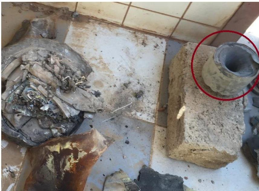
Figure 1.3 – Solid rocket motor venturi documented at Site YEM049 (IMG_4007).
