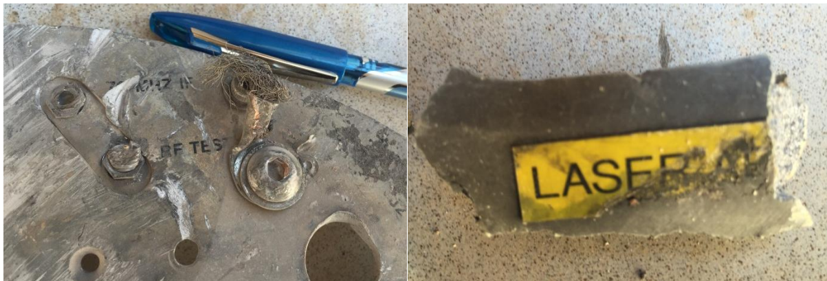
Left: Figure 1.5 – Structural baffle plate showing markings indicating an intermediate frequency of 70 MHZ documented at site YEM049 (IMG_3999).
