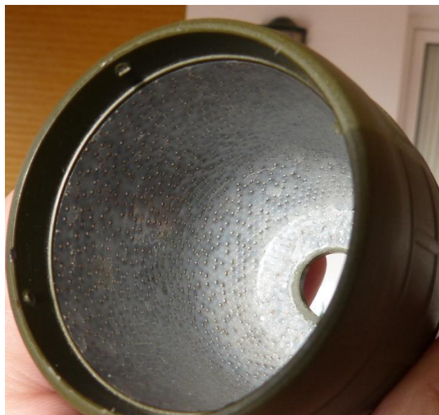
Figure 2.2 Internal view of an Alhambra D/O fragmentation shell, showing the pre-formed fragments (spheres) in the fragmentation matrix (source: original source unknown).
