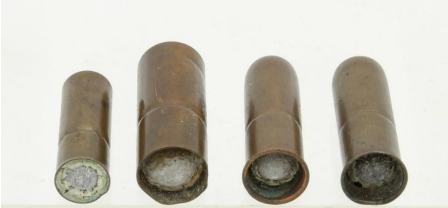
Figure 3.2 L–R: .28 Ellis & White cupfire; .42 Ellis & White cupfire; .32 Moore teatfire; .32 Moore-Williamson teatfire. Note that the projectiles are visible, recessed into their cases (source: Drake Watkins/ARES).
