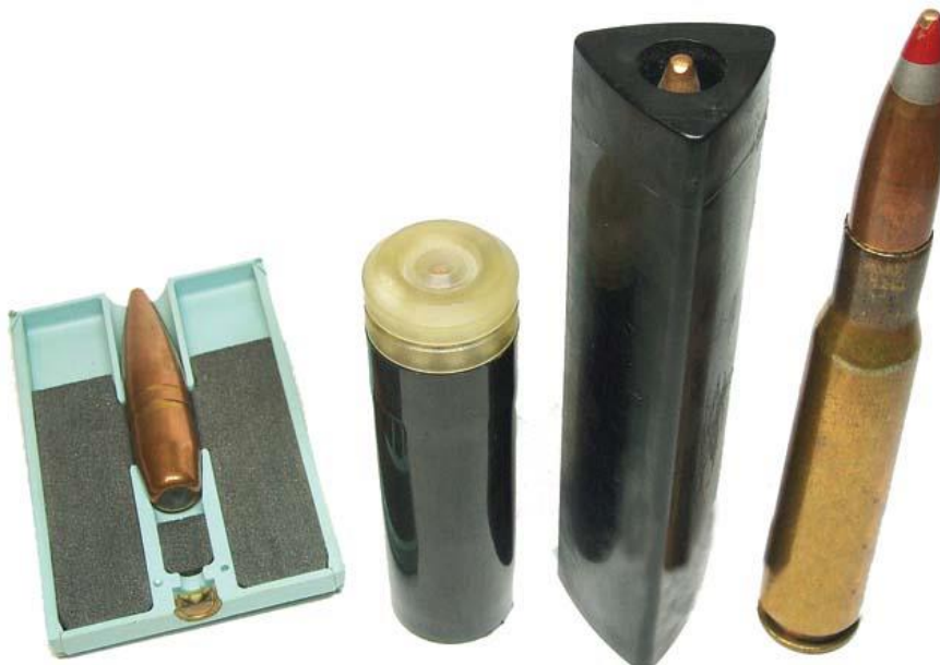
Figure 3.8 Experimental .50 calibre cartridges, L–R: Hughes Lockless, ARES TARG, Dardick Tround; .50 BMG (12.7 × 99 mm) for scale (source: Anthony G. Williams/SAR).
