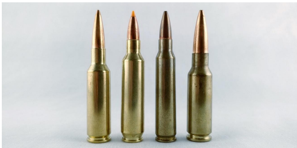
Figure 6.2 The .224 Valkyrie (far left) uses a much finer projectile shape and a heavier bullet than the 5.56mm (centre-right) to retain more energy over longer distances, despite being the same calibre. It is closer, ballistically-speaking, to the larger 6.5 Grendel round (far right), and even superior in some respects, despite being smaller in calibre (source: Nathaniel Fitch/ARES).
