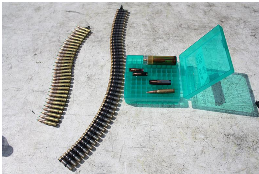
Figure 4.3 A belt of Textron's 5.56 mm CT ammunition on display at a demonstration. Sectioned ammunition illustrates the buried projectile (source: U.S. Army).
