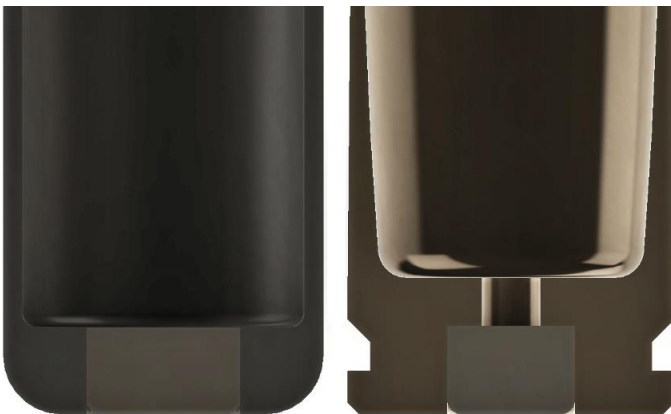
Figure 2.1 Sectioned polymer case heads compared. The cased telescoped configuration (left) lacks the substantial extractor groove cut of the conventional cartridge case (right) and is thereby stronger (source: Nathaniel Fitch/ARES).
