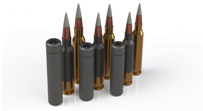
Figure 1.1 A suite of (L–R) 5.56 mm, 6 mm, and 6.5 mm cartridges each in (back to front) conventional brass cased, hybrid composite cased, and cased telescoped configurations (source: Nathaniel Fitch/ARES).
