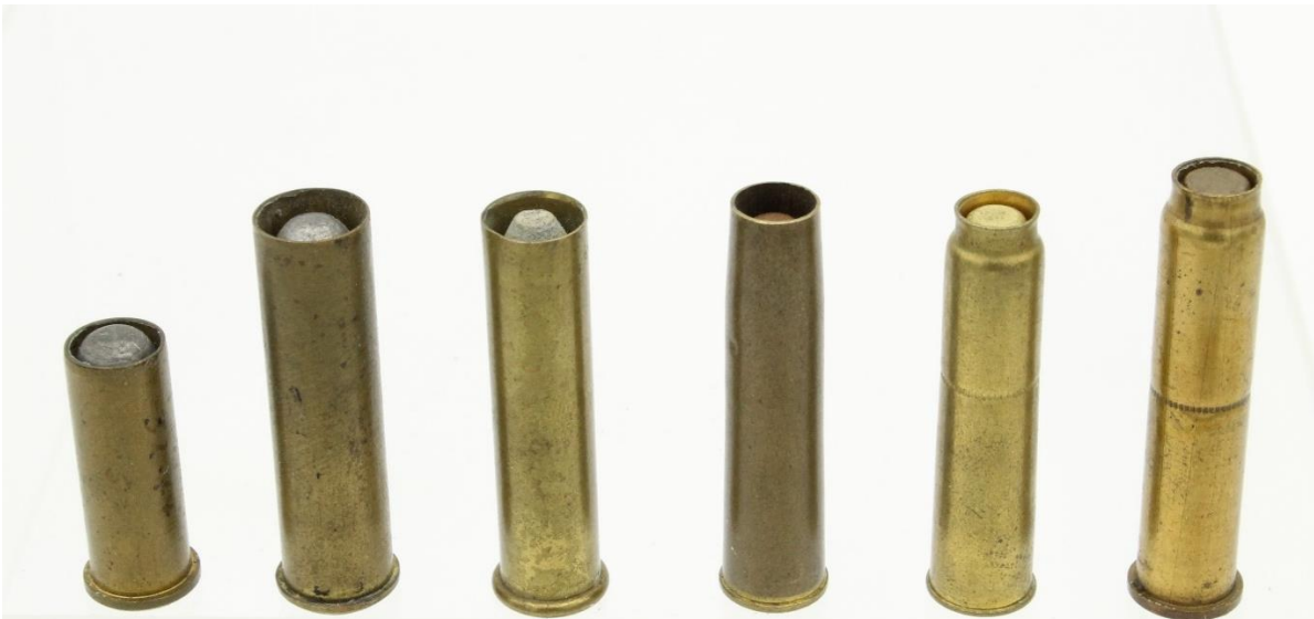
Figure 3.3 Semi-telescoped cartridges of the 19 th century. L–R: .32-44 S&W Target; .38-44 S&W Target; .32 S&W Rifle; 7.62 × 38R mm Nagant (military production); 7.62 × 38R mm Nagant (commercial production); 8 × 41R mm Pieper (source: Drake Watkins/ARES).
