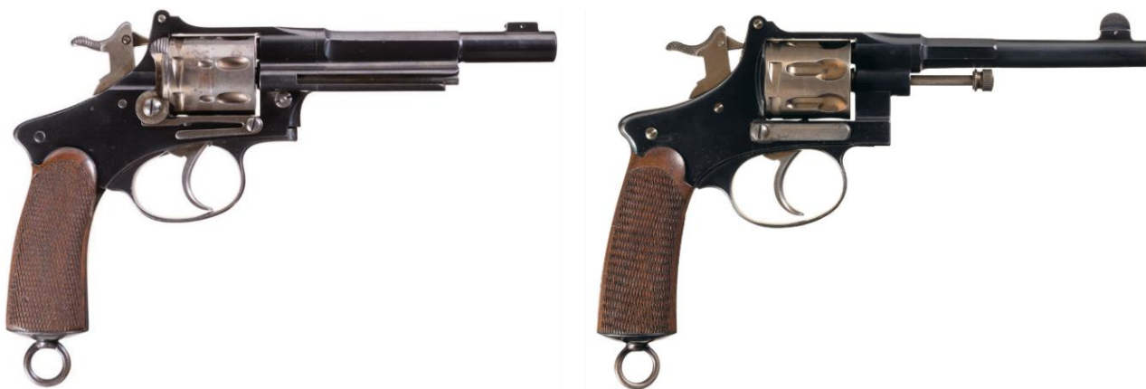
Figure 3.4 The Steyr (left) and Steyr-Pieper (right) revolvers as submitted to the 1897 Austrian military trials. Both are fitted with gas-seal mechanisms and are chambered for semi-telescoped cartridges, however the Steyr-Pieper has other improvements, including a swing-out cylinder and ejector rod (source: Rock Island Auction Company).
