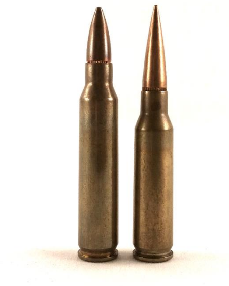
Figure 7.1 5.56 × 45 mm M193 (left) compared with 5.56 × 38 mm FABRL (right) (source: Nathaniel Fitch/ARES).
