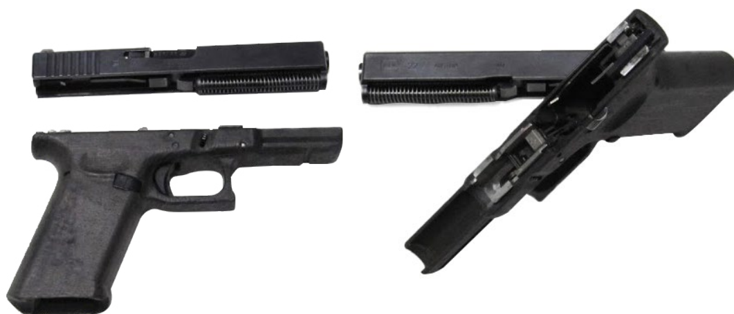
Figure 5.4 A Glock 17 frame printed in DuPont 'Zytel' glass-filled nylon. Factory Glock pistols use a near-identical polyamide 66 type material. Note the visible metal rails at right (source: Ivan T./ARES).
