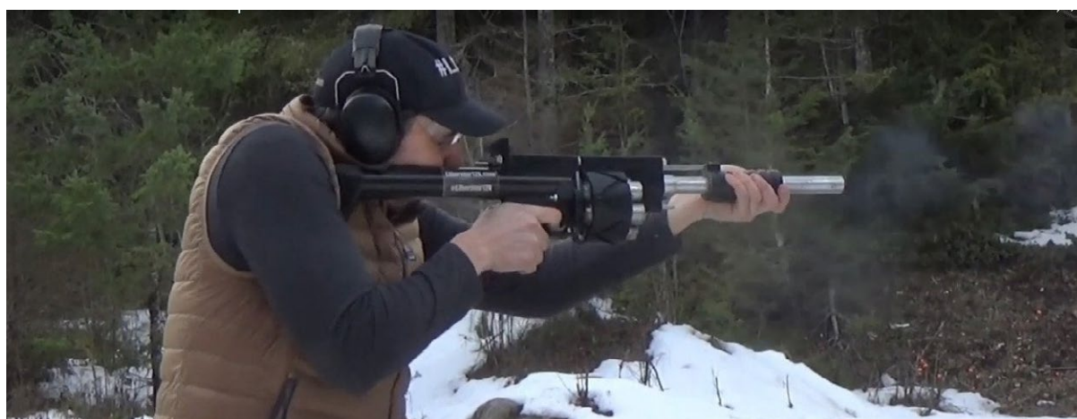
Figure 3.2 The ‘Liberator12k’ is a hybrid 3D-printed six-shot pump-action revolver shotgun. This design relies on thick-walled steel tube inserts and uses no original-purpose firearms components (source: Rodriguez, 2019).
