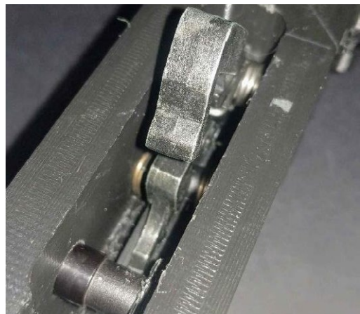
Figure 6.3 An airsoft trigger group fitted to a 3D-printed FGC-9 lower receiver (source: Ivan T./ARES).
