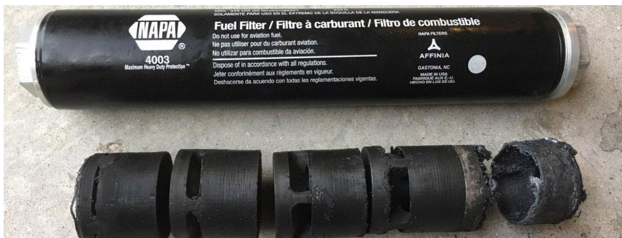
Figure 5.22 Printed baffles subjected to 150 rounds of continuous fire using .223 Remington ammunition (source: KadeCAD).
