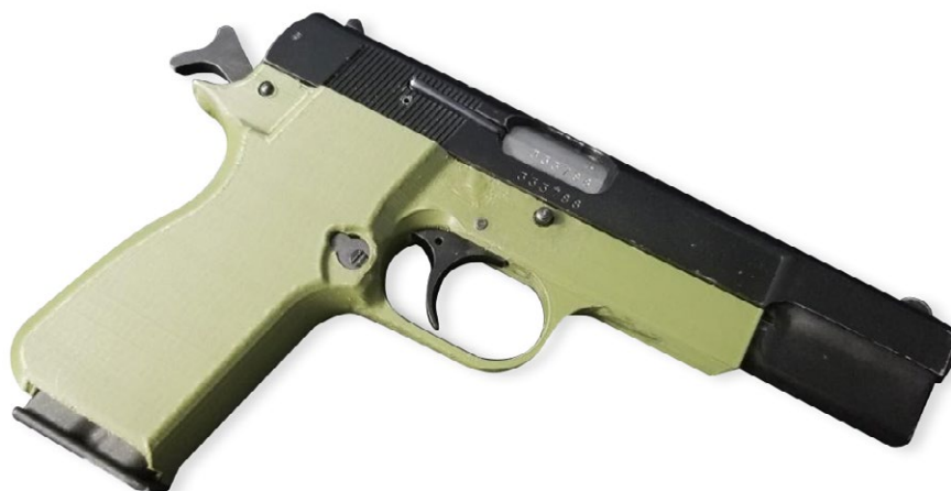
Figure 5.9 A Browning Hi-Power self-loading pistol with a 3D-printed frame (source: Ivan T./ARES).
