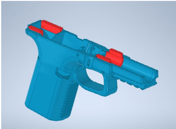
Figure 5.5 CAD diagram showing the placement of metal rail inserts (red) in the 3D-printable Glock 17 receiver (source: Ivan T./ARES).
