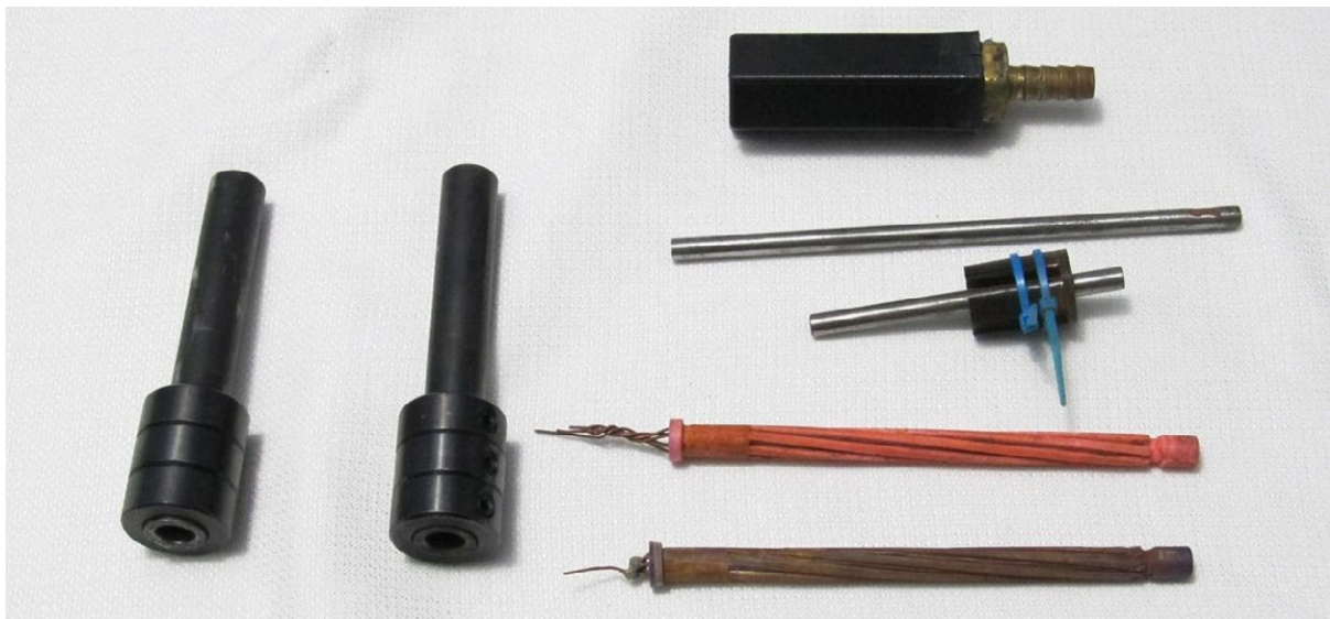
Figure 5.18 Two finished FGC-9 barrels (left) and the 3D-printed cathodes, jigs, and materials used (right) (source: Ivan T./ARES).
