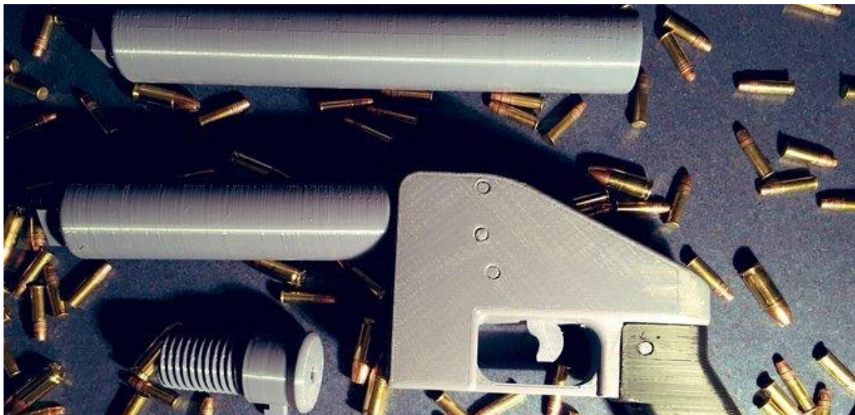
Figure 5.23 A modified .22 LR version of the Defense Distributed Liberator fitted with an experimental printed barrel and removeable suppressor unit (source: KadeCAD).
