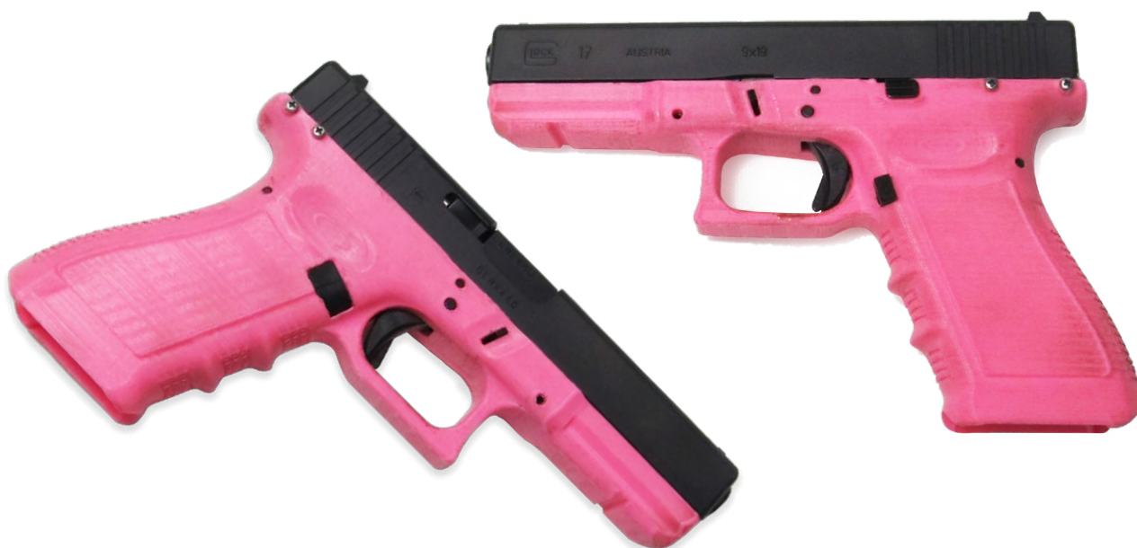
Figure 1.1 A Glock 17 pistol with a 3D-printed (pink) polymer frame (source: Ivan T./ARES).
