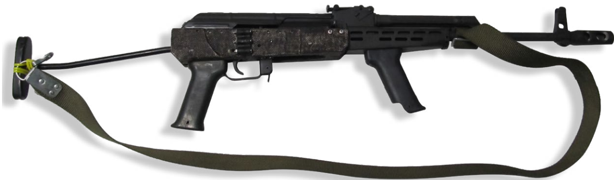
Figure 5.7 The 'Plastikov', a 3D-printable AKM pattern receiver recently developed by IvanTheTroll. The example pictured is assembled using Hungarian AMD parts (source: Ivan T./ARES).
