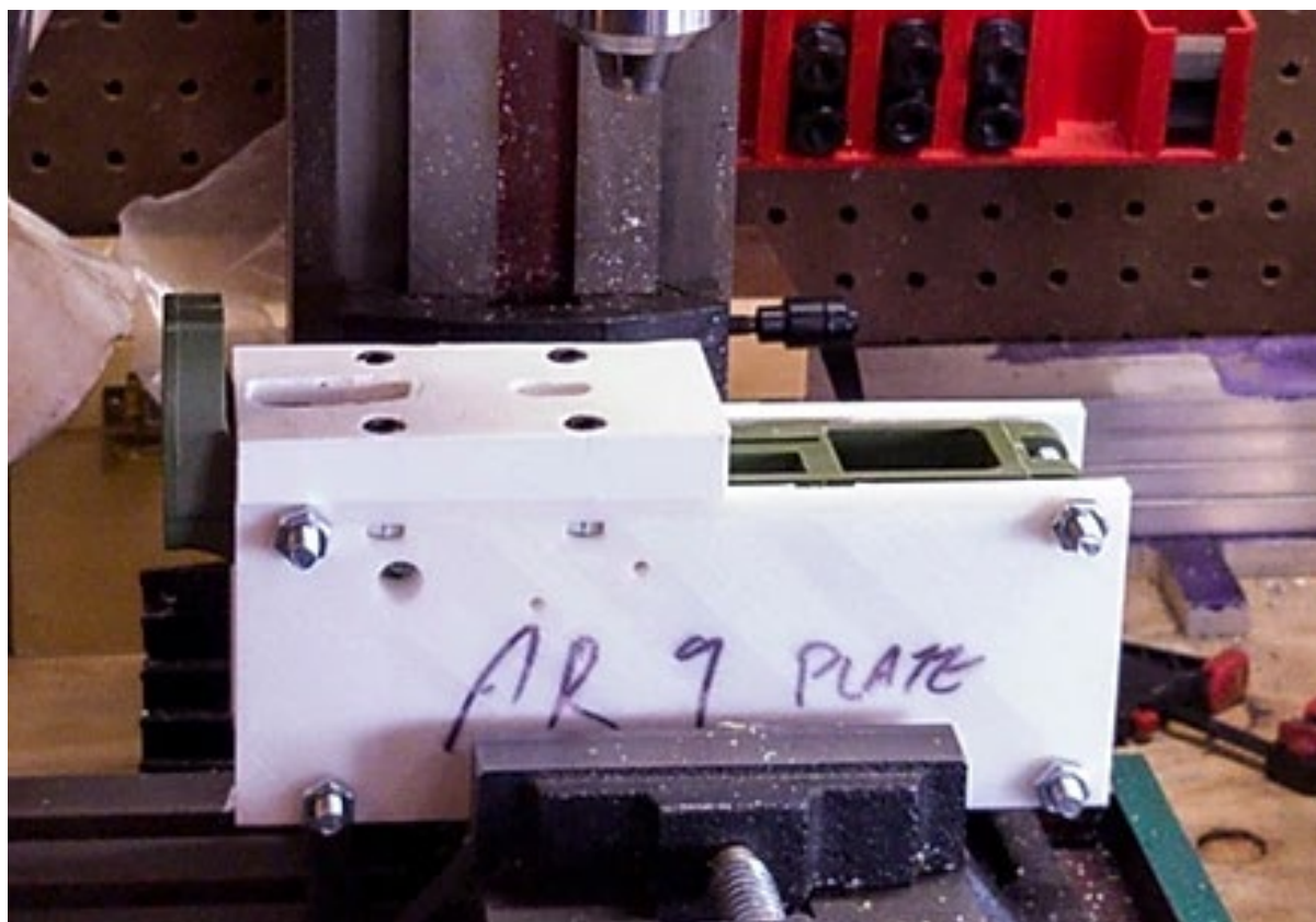
Figure 5.24 A 3D-printed receiver milling jig for AR-15-type ‘80% lowers’ (source: Ctrl+Pew).
