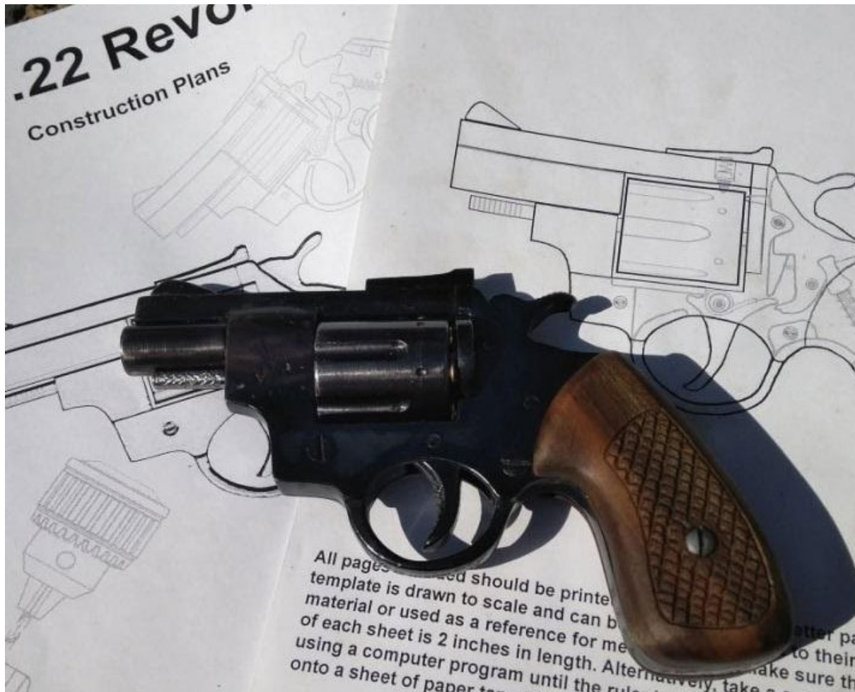
Figure 4.2 A .22 LR calibre revolver, made using traditional craft production techniques and based upon widely available construction plans. The skill level required to produce this sort of craft-produced firearm is higher than for some 3D-printed designs (source: ImproGuns).
