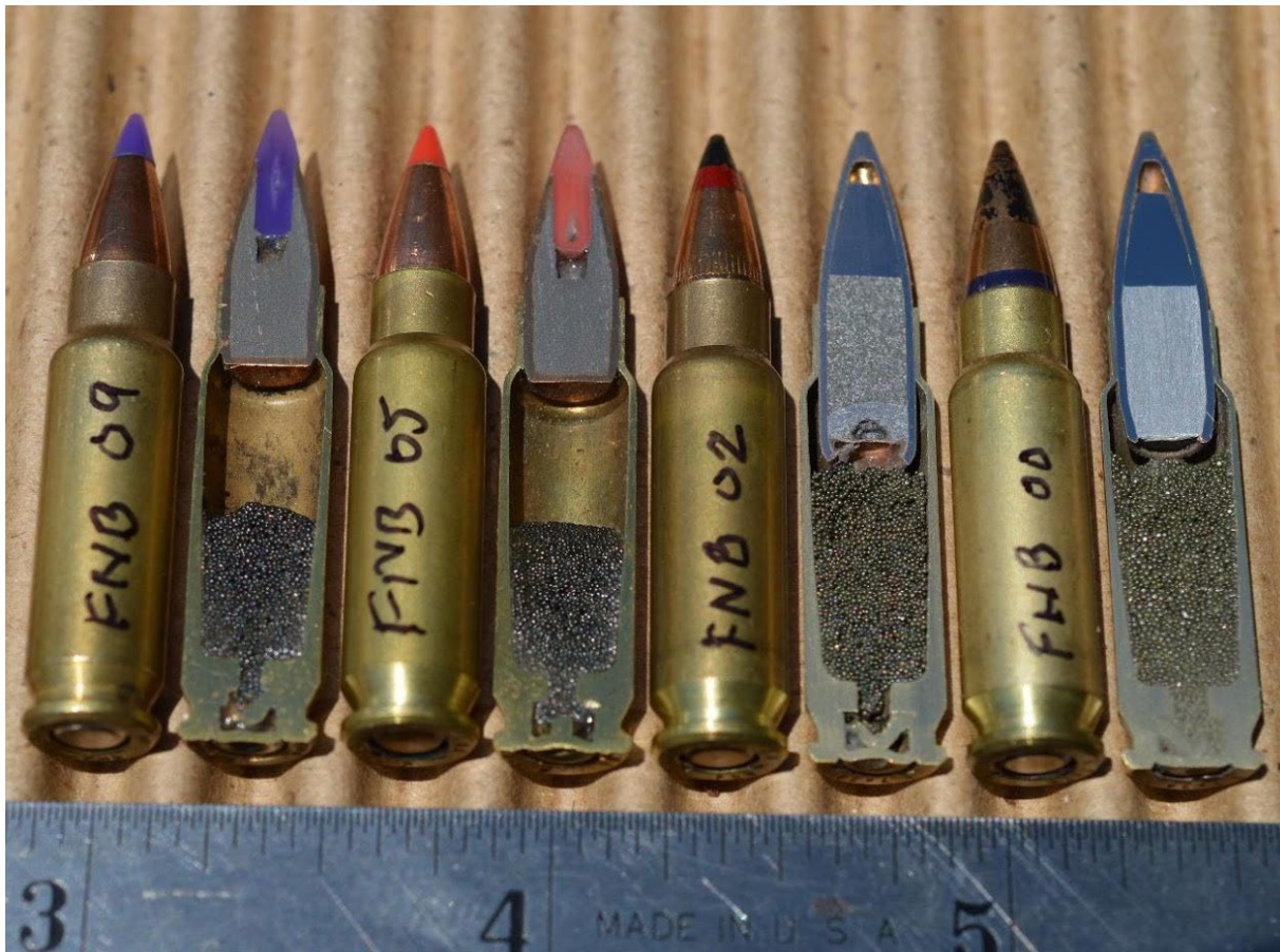
Figure 2.2 Sectioned examples of selected 5.7 × 28 mm cartridges; a.) SS197SR, b.) SS196SR, c.) L191, d.) SS190. Note the aluminium core (rear) and steel penetrator (forward) in the SS190 round, and the hollow-point design with ballistic tip of the two sporting rounds (source: Wolfgang Gross).
