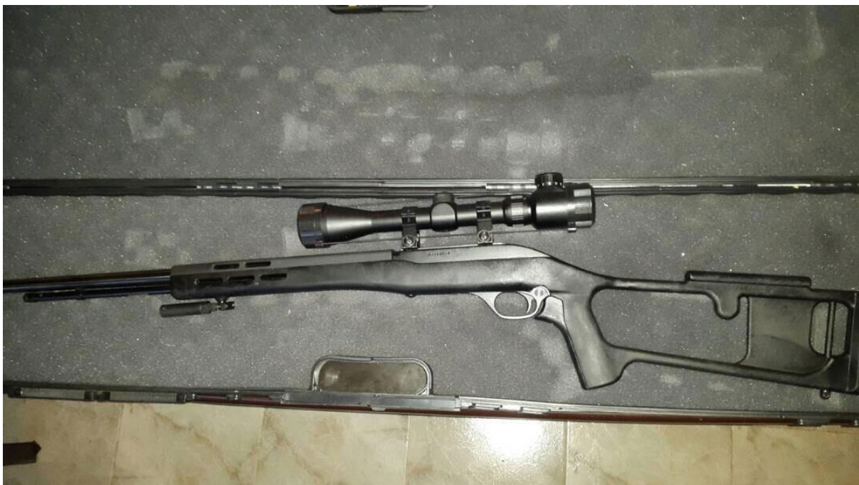
Figure 4.29 A Marlin Model 60 self-loading rifle (.22LR), fitted with scope and mounted in an aftermarket polymer chassis with thumbhole style butt-stock (source: ARES CONMAT Database).
