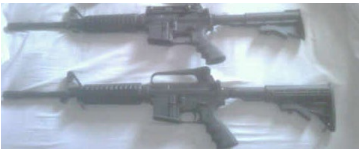
Figure 4.15 Two generic M4-style AR-15-type self-loading rifles, both with longer (16-inch) barrels than the military equivalent (14.5 in) and both fitted with non-standard 'ergonomic' pistol grips. The bottom example also has the older style fixed carrying handle; not present on issue USGI M4 rifles (source: ARES CONMAT Database).
