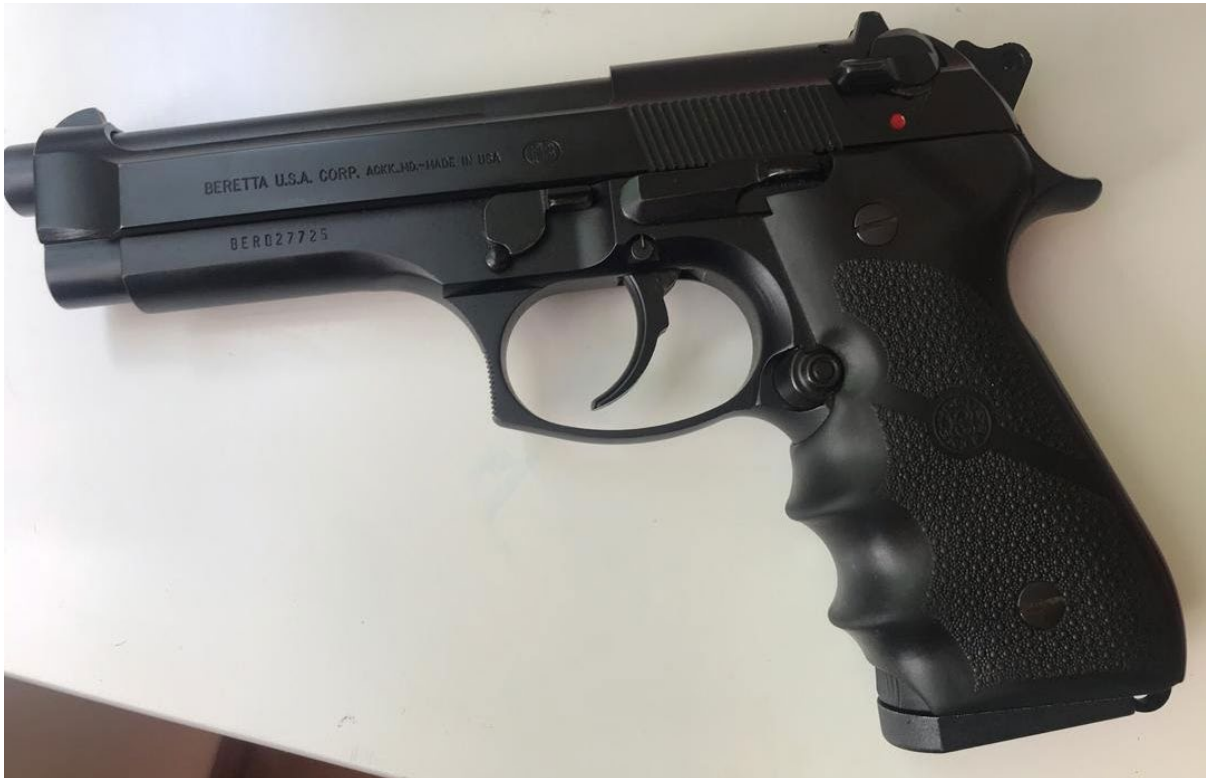
Figure 4.10 A US-made Beretta 92FS handgun. Note the US manufacturer markings and the distinct ‘BER’ serial number prefix used only on US-made firearms. The serial number indicates the weapon was produced in 1997 (source: ARES CONMAT Database).
