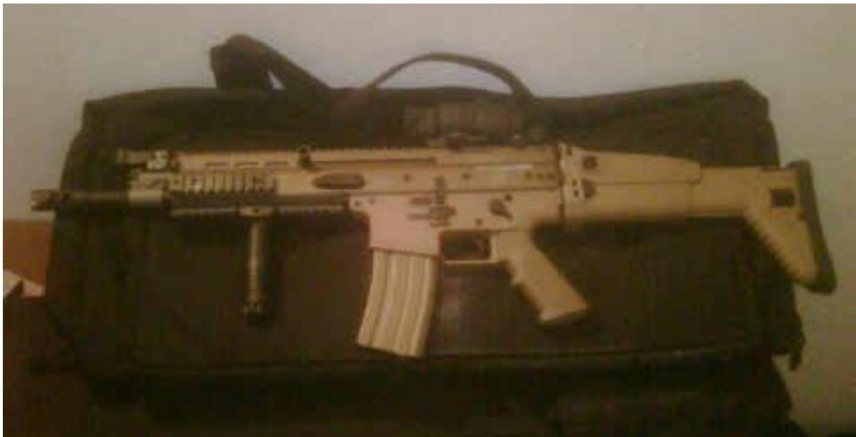
Figure 4.26 FN Herstal SCAR-L self-loading rifle, chambered for 5.56 × 45 mm (source: ARES CONMAT Database).
