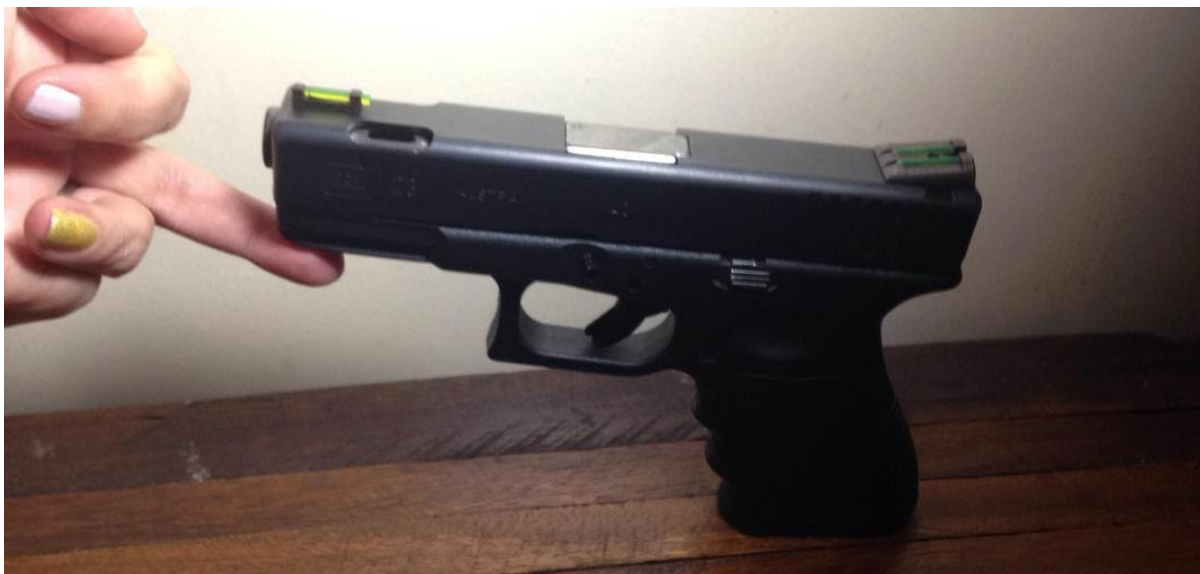
Figure 4.4 A Gen3 Glock 23 (.40 S&W) compact self-loading pistol with ported barrel and slide and aftermarket fibre optic sights (source: ARES CONMAT Database).
