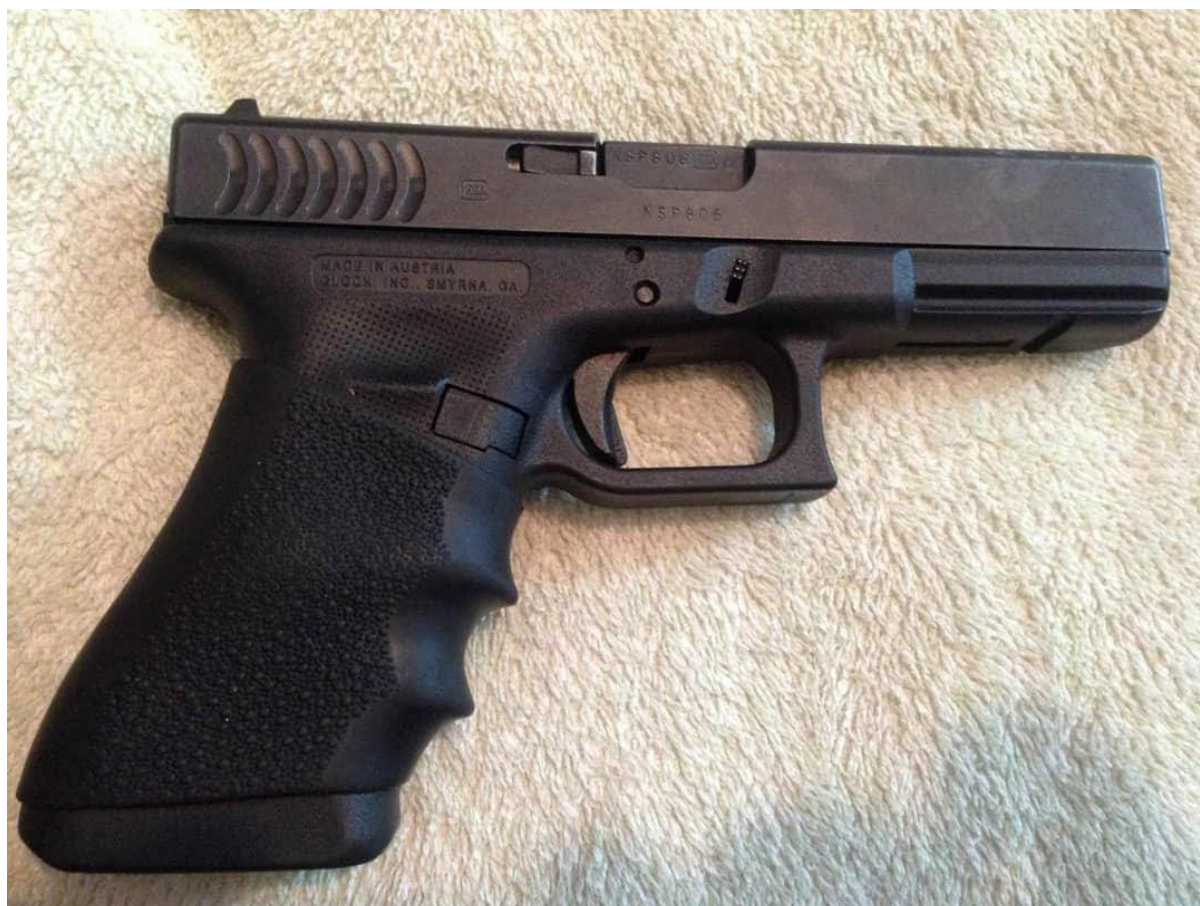
Figure 4.3 A U.S.-made Gen3 G17 fitted with a Hogue 'HandALL' aftermarket grip sleeve. Note the clear manufacturer's markings for Glock's Smyrna, Georgia plant. The curved 'fish-gill' slide serrations denote a rare variant of the Gen3 pistol with the RTF2 frame texture (source: ARES CONMAT Database).
