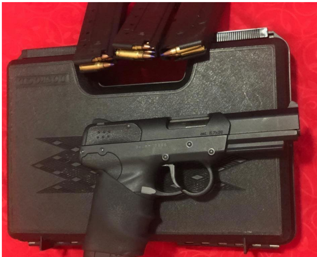
Figure 4.11 One of three FN Herstal Five-seveN pistols offered for sale. Both early (curved trigger guard, as here) and late (straight guard) types were represented. Note the prominent blue ballistic tips of the SS197SR 5.7 × 28 mm ammunition. Despite this, the cartridges were described by the seller as “armour-piercing” (source: ARES CONMAT Database).
