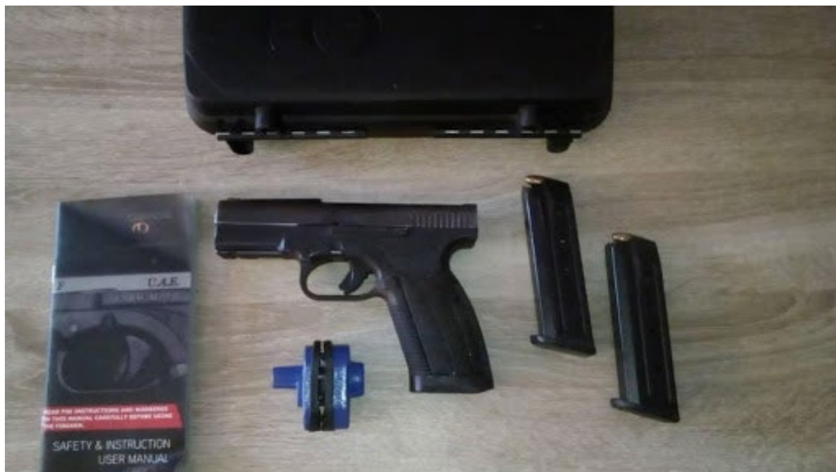
Figure 4.13 An as-new Caracal F self-loading pistol (9 × 19 mm) with case, three magazines, user manual and even its manufacturer-supplied trigger lock device. Note that this model is fitted with Caracal's proprietary 'Quick Sight' system, a point-shooting sight reminiscent, in some respects, of the ASP 'Guttersnipe' sights (source: ARES CONMAT Database).
