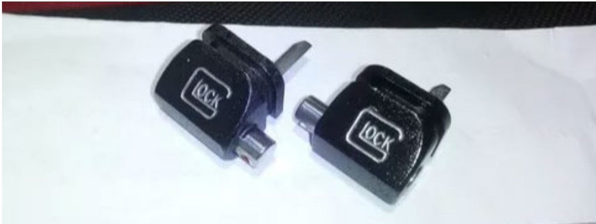
Figure 3.13 Two craft-produced selector backplates for Glock pistols, with black finish and spurious Glock markings. The large cross-bolt is pressed to the left for automatic fire, right for semi-automatic (source: ARES CONMAT Database).
