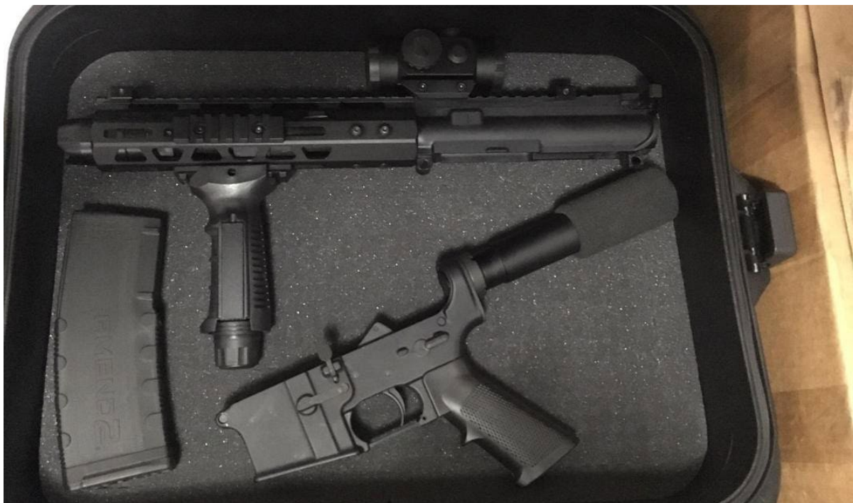
Figure 4.19 An AR-15 'pistol' build with completely unmarked lower receiver, one of a number likely produced from '80%' lower receivers (source: ARES CONMAT Database).
