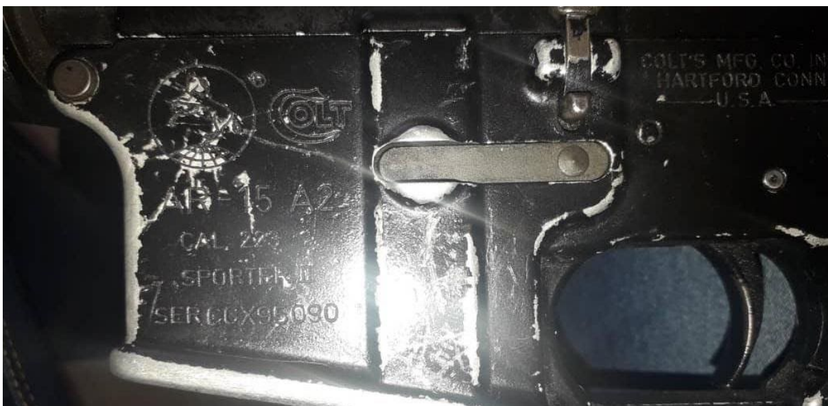
Figure 4.21 Also from the dataset, a genuine Colt AR-15A2 Sporter II with correct markings, valid serial number, and in original factory configuration (source: ARES CONMAT Database).
