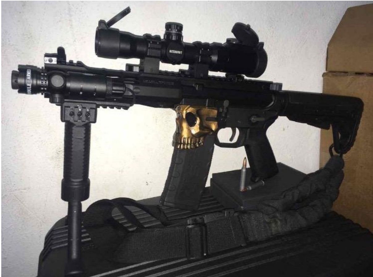
Figure 4.23 This 'AR' build incorporates a skull-shaped lower receiver known as 'The Jack', designed and produced by Spikes Tactical/Sharps Bros in the United States. Like many others in the dataset, it is festooned with accessories (source: ARES CONMAT Database).
