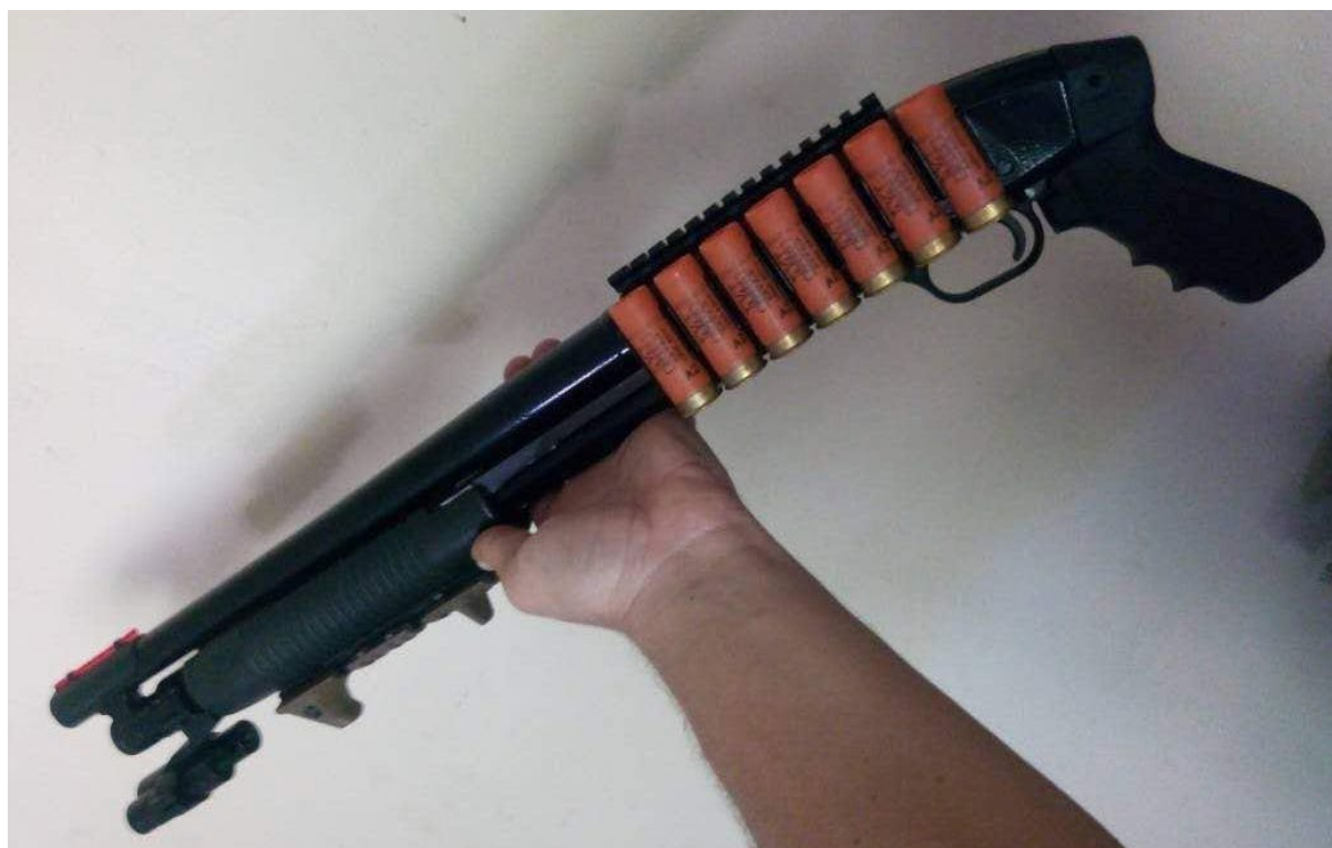
Figure 4.30 One of many 12 gauge pump-action Mossberg shotguns in the dataset, in this case a Model 500 with pistol grip, short barrel, ‘Picatinny’ top rail, 6 o’clock railed pump grip fitted with ‘hand-stop’ accessories, a ‘side-saddle’ shell holder, fibre-optic front sight, and laser aiming unit (source: ARES CONMAT Database).
