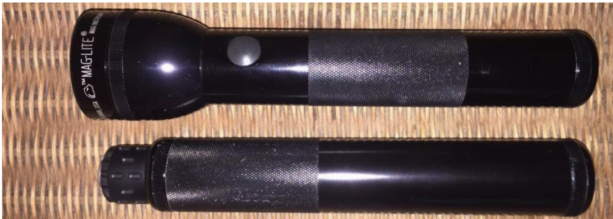
Figure 3.10 A suppressor improvised from a Maglite torch body, with a similar Maglite model for comparison (source: ARES CONMAT Database).
