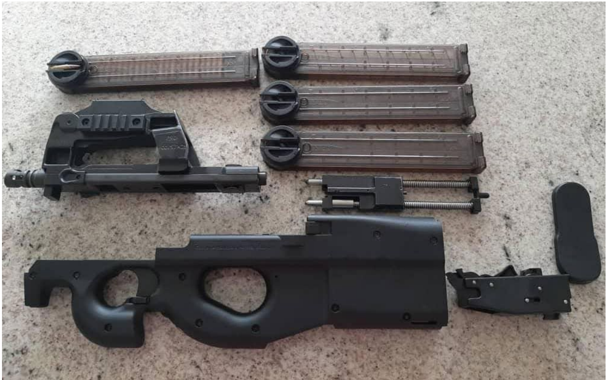
Figure 4.37 The single FN P90 SMG (5.7 × 28 mm) shown in disassembled state with four magazines (source: ARES CONMAT Database).
