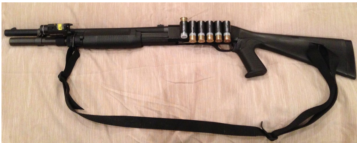
Figure 4.33 A Benelli M3 Super 90 dual-mode (pump-action and semi-automatic) shotgun, fitted with a Streamlight TLR-2 tactical light with integrated red aiming laser, on a CDM gear picatinny rail mount, TacStar side-saddle shell carrier, and Blackhawk! sling (source: ARES CONMAT Database).
