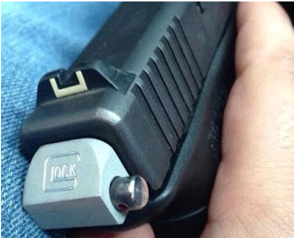
Figure 3.14 An 'in-the-white' selector shown fitted to a pistol (source: ARES CONMAT Database).
