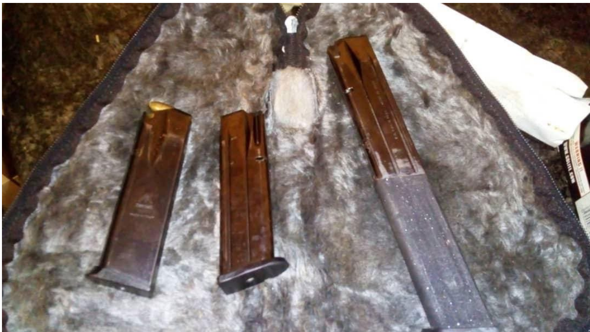
Figure 3.17 A locally produced extended magazine, known as a 'Cocostette', which is made by welding together two 17-round 9 x 19 mm magazines for the Beretta Px4. Demand for this modification may be due to the fact that there are no commercially manufactured magazines for the Beretta Px4 that have a higher capacity than 20 rounds. (source: ARES CONMAT Database).
