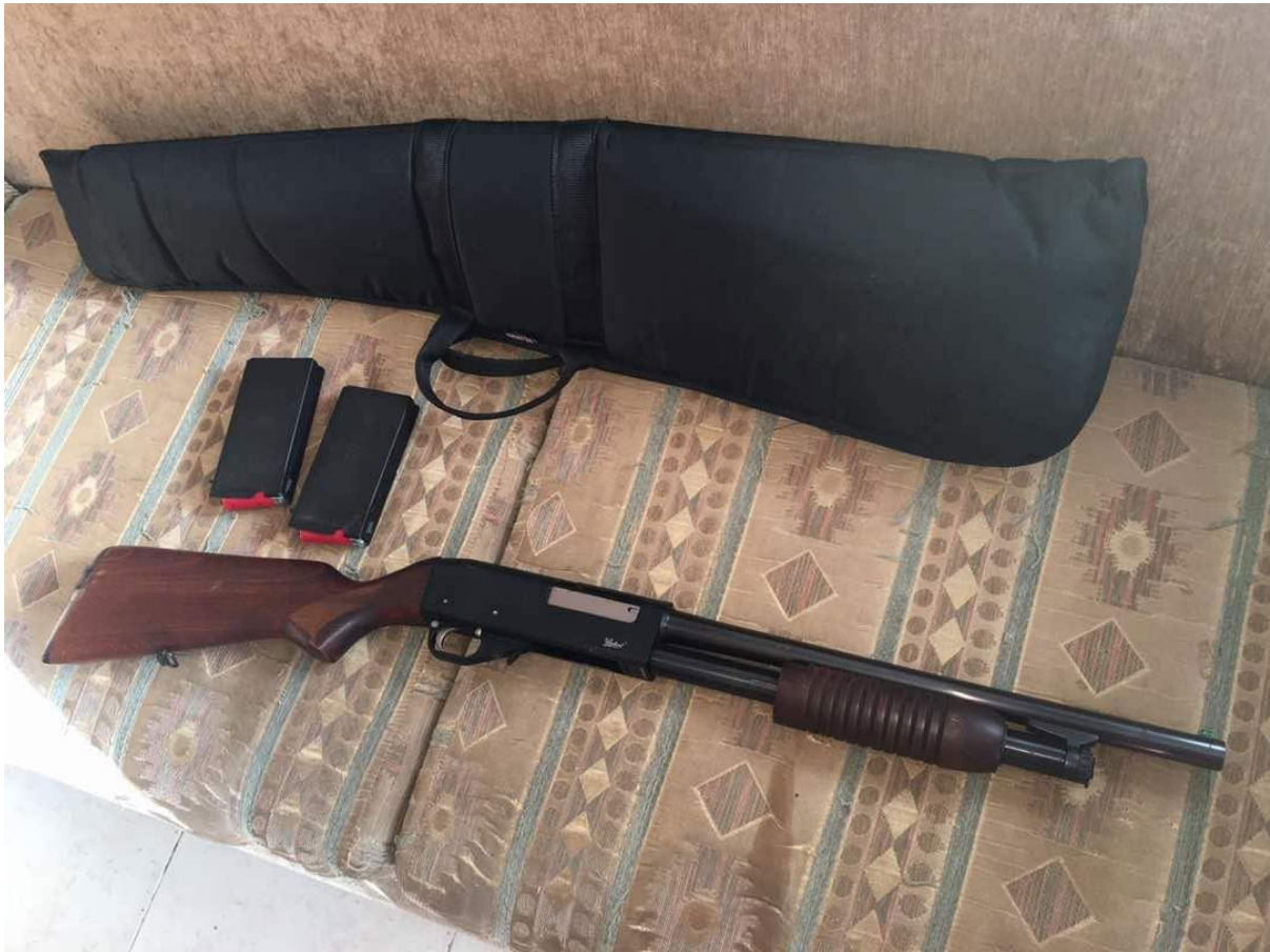
Figure 4.34 A Russian Baikal IZH-81KM 12-gauge pump-action shotgun fed from detachable box magazines (source: ARES CONMAT Database).
