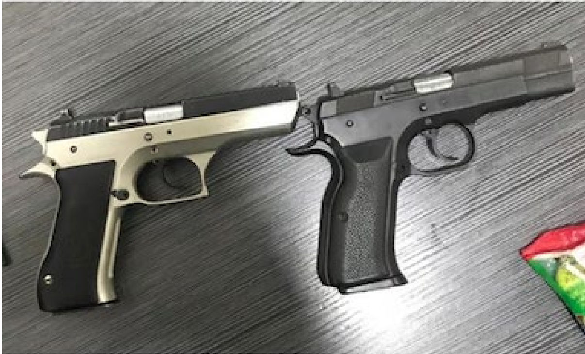
Figure 4.12 Two derivatives of the Czech CZ 75 from the dataset: an IMI/IWI Jericho (left) and a Tanfoglio T95 (right) (source: ARES CONMAT Database).
