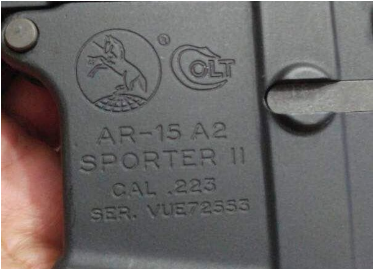
Figure 4.20 A spuriously marked lower receiver, purporting to be a Colt 'AR-15A2 Sporter II'. Amongst other incongruous features, the Colt logo is a crude copy of the genuine version (source: ARES CONMAT Database).
