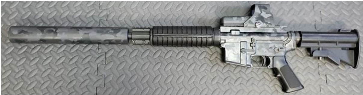
Figure 3.9 An AR-15-type self-loading rifle fitted with a large sound suppressor. The rifle, suppressor, and an EOTech-type holographic sight have all been finished with a camouflage pattern. The rifle has been built with a low-profile gas block lacking the classic AR-15 triangular front sight structure (source: ARES CONMAT Database).
