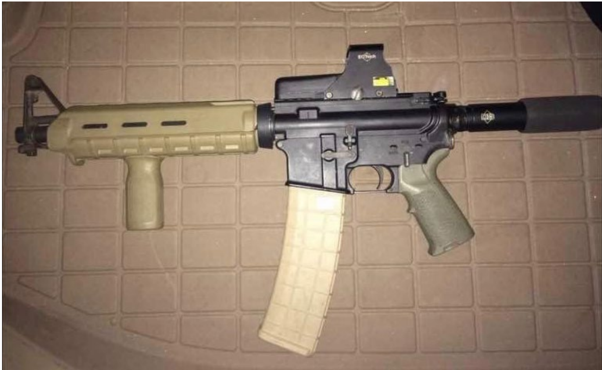
Figure 4.17 AR-15 rifle in a U.S.-legal 'pistol' configuration built on a Diamondback DB-15 lower receiver with Magpul furniture and a 'Drum Magazines' 42-round box magazine. 37 The barrel lacks a muzzle device or any visible threading, suggesting that it may have been cut down (source: ARES CONMAT Database).
