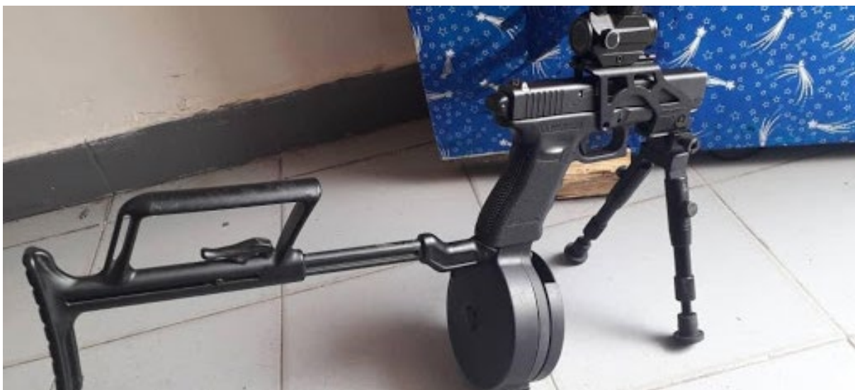
Figure 3.11 An elaborately accessorised and highly impractical Generation 3 Glock 17 self-loading pistol fitted with selector backplate, optical sight mount, Primary Arms Microdot series red dot sight, rifle bipod, FAB Defense shoulder stock, and 50-round drum magazine from SGM Tactical (source: ARES CONMAT Database).
