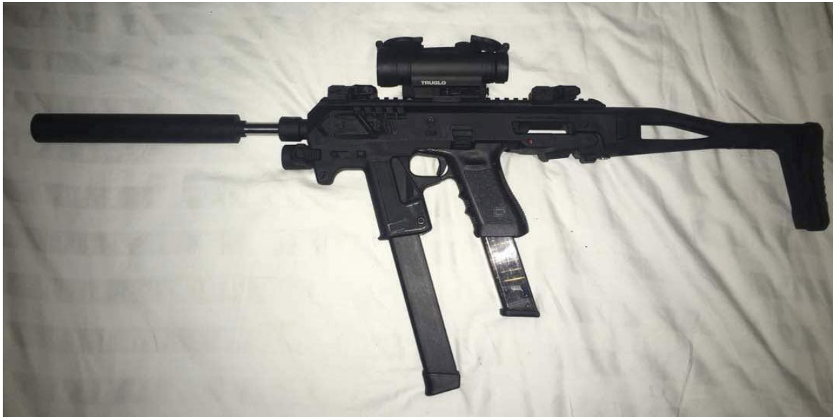
Figure 4.7 A Gen3 Glock 17 fitted into a CAA Roni stock/chassis and further accessorised with extended barrel, sound suppressor, Truglo optical sight, extended ETS magazine, and 33-round spare magazine (source: ARES CONMAT Database)
