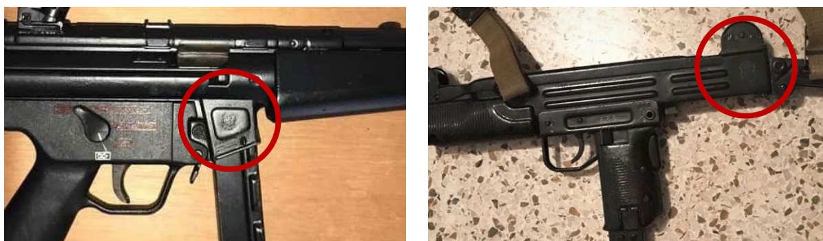
Figure 3.2 Visible national crest markings—circled in red—on MP5 (left) and Uzi (right) sub-machine guns. These weapons are likely to have been stolen from the armouries of security services, or captured from military or law enforcement personnel (source: ARES CONMAT Database).
