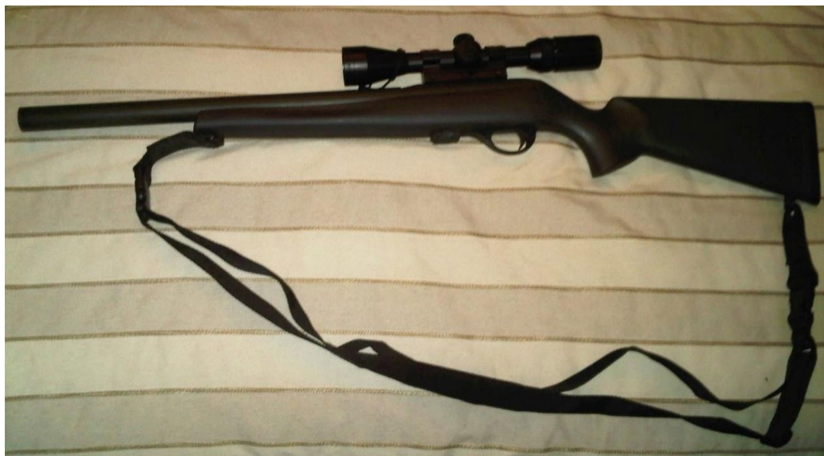
Figure 3.8 An integrally suppressed Remington Model 597 self-loading rifle chambered for .22 LR (source: ARES CONMAT Database).
