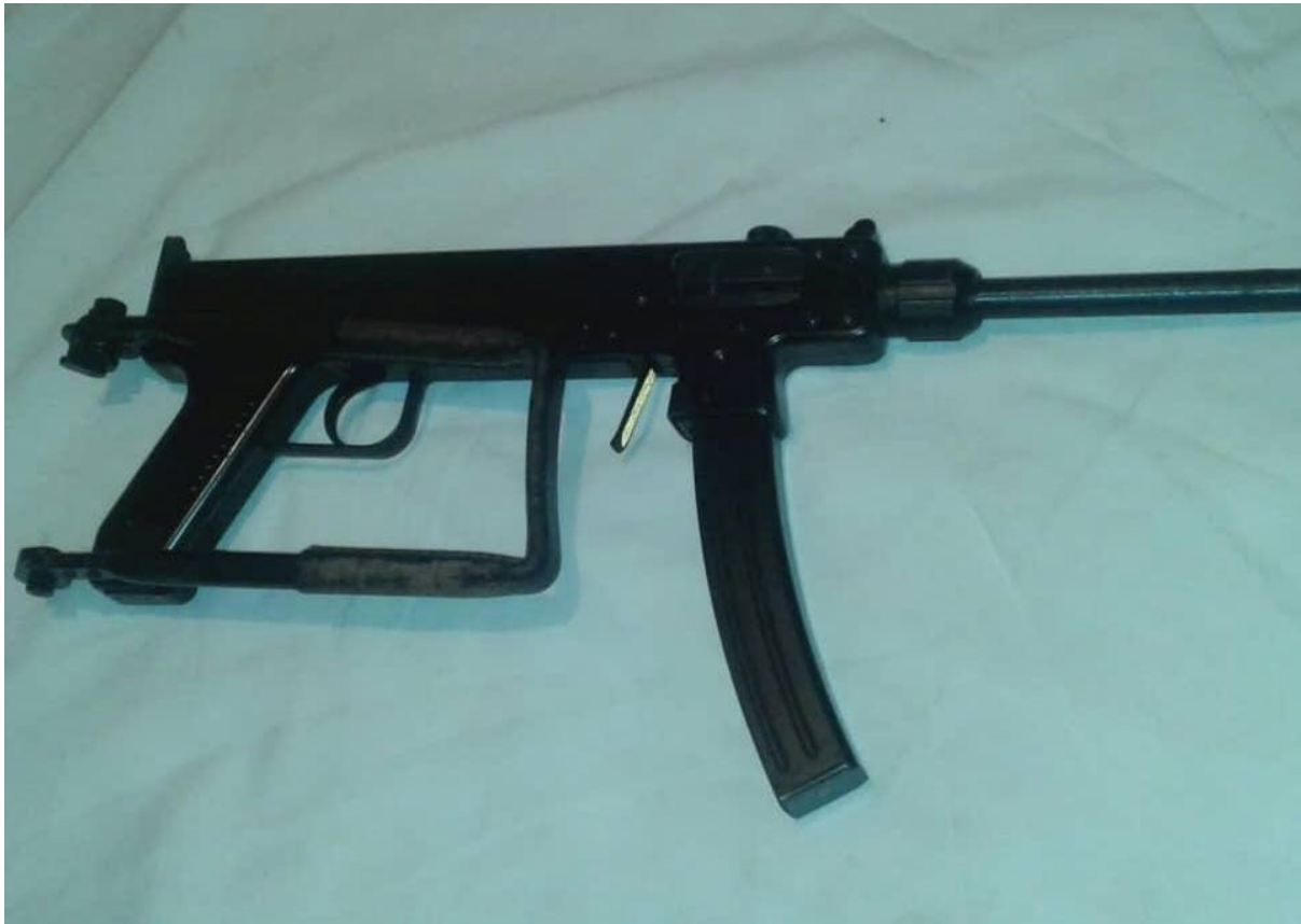
Figure 4.36 A Danish Dansk Industri Syndikat Madsen M50 SMG, chambered for 9 × 19 mm (source: ARES CONMAT Database).
