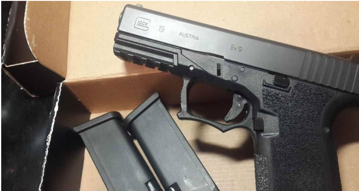
Figure 3.15 A Glock pattern self-loading pistol built on a Polymer 80 ‘80% lower’ frame, mounting a pre-Gen4 (likely Gen3) slide assembly. The (grooved, U.S. pattern) trigger, disassembly catch, slide lock and magazine release are standard Gen3 Glock pattern components, readily available online (source: ARES CONMAT Database).
