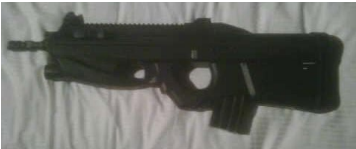
Figure 4.27 FN Herstal FS2000 self-loading rifle, chambered for 5.56 × 45 mm (source: ARES CONMAT Database).
