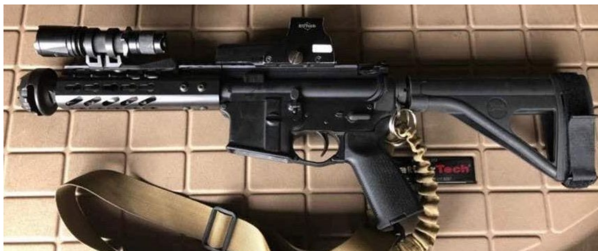
Figure 4.16 AR-15 rifle in a U.S.-legal 'pistol' configuration, pictured with the SOB arm brace produced by U.S. firm SB Tactical, as well as a Strike Industries 'cookie cutter' muzzle brake (or Chinese copy), Keymod modular handguard with flashlight and mount, EOTech reflex sight, MOE pistol grip (or clone) and single-point sling (source: ARES CONMAT Database).
