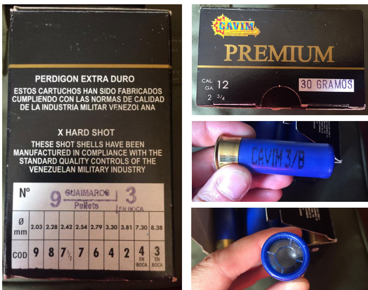
Figure 4.20 A box of 25 CAVIM Premium #3 buckshot cartridges. Each cartridge contains nine pellets weighing a total of 30 g (source: ARES).
