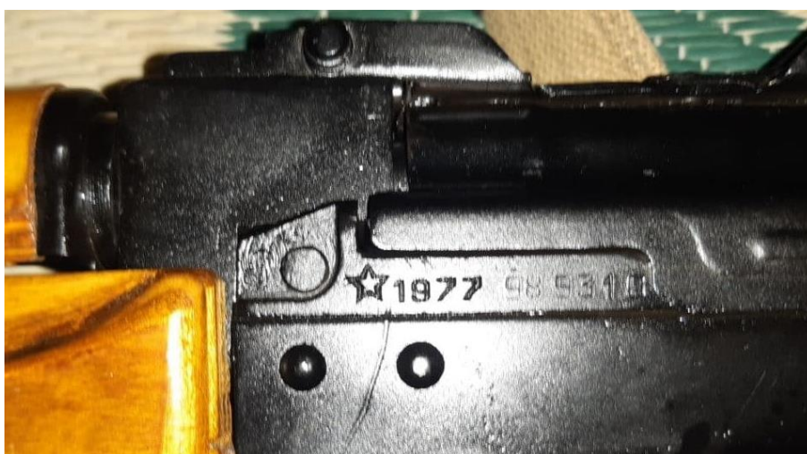
Figure 2.4 Trunnion markings on an AKM converted to look like an AKS-74U, indicating it was produced at Tula in the Soviet Union in 1977 (Source: ARES CONMAT Database).
