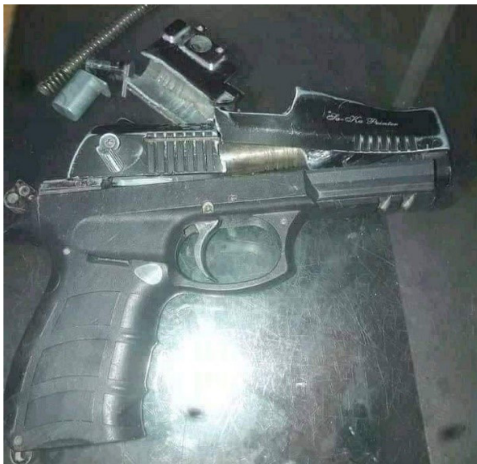
Figure 2.12 A Turkish Aksa Silah AK15 blank-firing pistol which has been converted to be capable of firing lethal-purpose cartridges, and subsequently experienced a catastrophic failure (source: ARES CONMAT Database).
