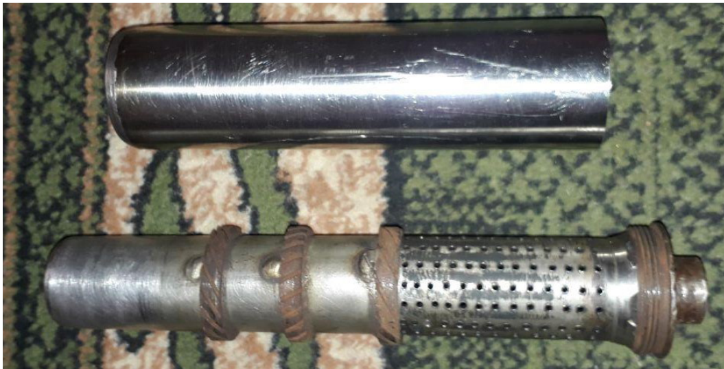
Figure 2.1 An Idlib-pattern craft-produced suppressor for sale in September 2019, with the internal components exposed (Source: ARES CONMAT).
