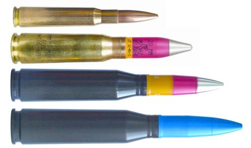
**Figure 2.7** Three common 20 mm cartridges compared with a common .50 inch (12.7 mm) cartridge. The former are used in light cannon, whilst the latter is used in heavy machine guns and some large rifles. Left to right: 12.7 × 99 mm, 20 × 102 mm, 20 × 128 mm, 20 × 139 mm (source: Nammo).
