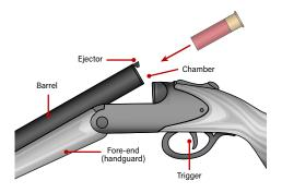
**Figure 2.38** A break-open firearm, in this case a shotgun, depicted with the action open (source: ARES).
