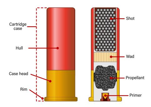
**Figure 2.16** Cross-sectional diagrams showing key components of a contemporary shotgun cartridge, in this case a 12-gauge (18.5 mm) shotgun cartridge (source: ARES).
