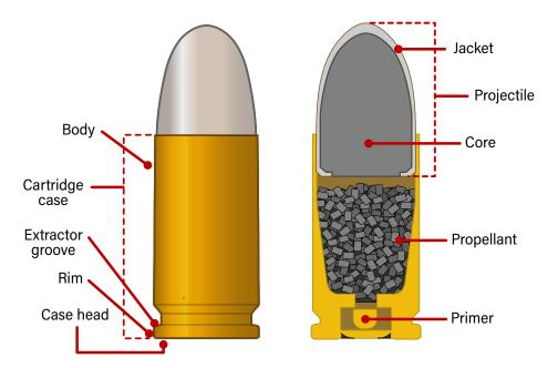
**Figure 2.15** Cross-sectional diagram showing key components of a contemporary handgun cartridge, in this case a  $9 \times 19$  mm cartridge (source: ARES).
