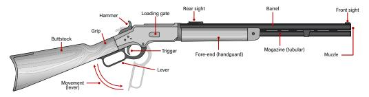
Figure 2.30 Typical parts of a lever-action rifle (sources: ARES).
