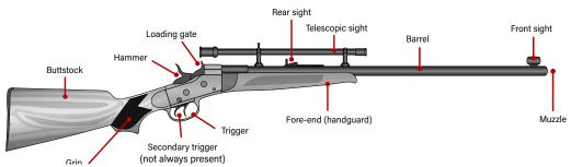
**Figure 2.28** Typical parts of a single-shot rifle, in this case fitted with an older style of telescopic sight (sources: ARES).
