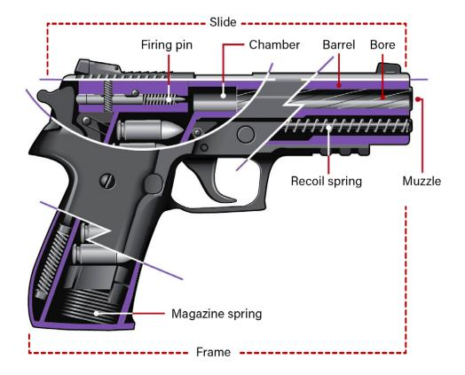
**Figure 2.43** A cutaway diagram of a typical self-loading pistol, in this case a semi-automatic example (sources: Small Arms Survey).
