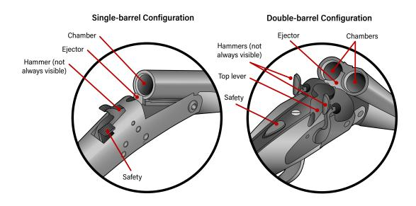
**Figure 2.22** Detail diagrams showing typical features of break-open shotguns, with the actions open. Left: a single-barrel design; right: a side-by-side, double-barrel design. Note that not all break-open shotguns have external hammers (see Figure 2.21, an over-and-under, double-barrel design with internal hammers) (sources: ARES).
