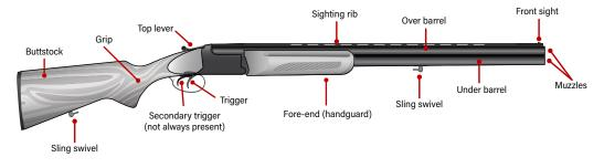
**Figure 2.21** Typical parts of a break-open shotgun, it this case a over-and-under, double-barreled shotgun (sources: ARES).
