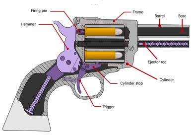
Figure 2.42 A cutaway diagram of a typical revolver (source: ARES).
