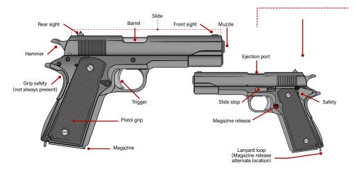
Figure 2.10 Typical parts of a self-loading pistol (sources: ARES).
