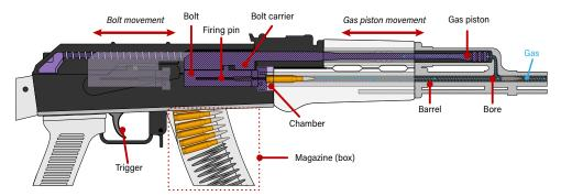
**Figure 2.44** A cutaway diagram of a typical self-loading rifle, in this case a gas-operated, selective-fire example (source: ARES).
