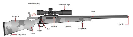
**Figure 2.29** Typical parts of a bolt-action rifle, in this case fitted with modern style of telescopic sight (sources: ARES).
