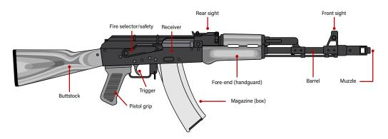
**Figure 2.31** Typical parts of a self-loading rifle, in this case a select-fire design with a detachable box magazine (sources: ARES).
