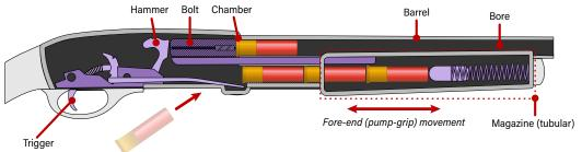
Figure 2.41 A cutaway diagram of a typical pump-action shotgun (source: ARES).
