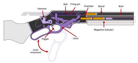
Figure 2.40 A cutaway diagram of a typical lever-action rifle (source: ARES).
