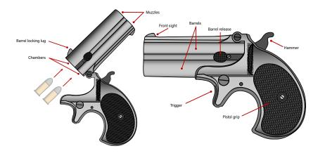
**Figure 2.8** Typical parts of a break-open handgun, in this case a double-barreled derringer (sources: ARES).
