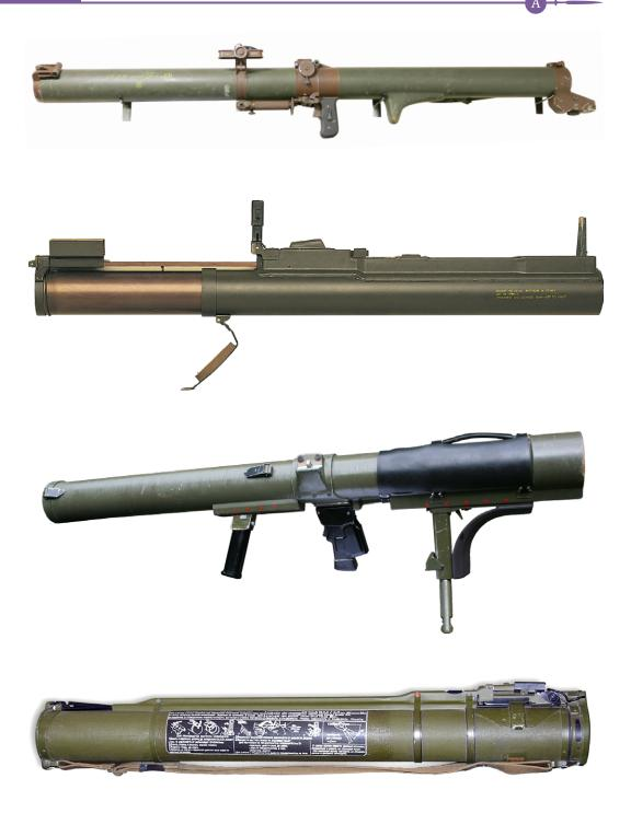
**Figure 2.56** Top to bottom: Mecar RL-83 Blindicide (Egyptian contract; 83 mm), Talley Industries M72A3 LAW (66 mm), MAS LRAC F1 (89 mm), NPO Bazalt RPG-18 (64 mm) [not to scale] (sources: N.R. Jenzen-Jones/ARES; Small Arms Survey; Zonawar).
