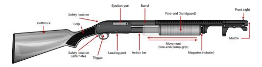
Figure 2.23 Typical parts of a pump-action shotgun (sources: ARES).
