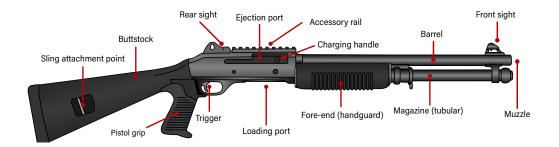
Figure 2.24 Typical parts of a self-loading shotgun (sources: ARES).
