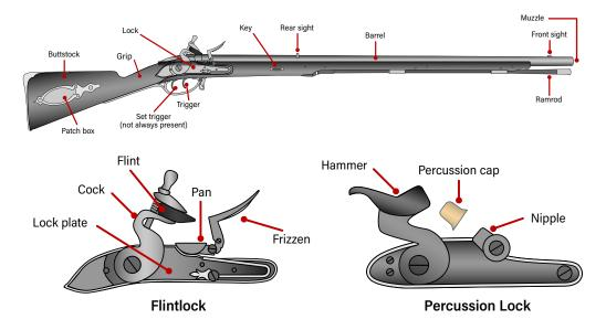
**Figure 2.45** Typical parts of a muzzle-loading firearm. Two common lock types, a flintlock and percussion lock, are depicted (sources: ARES).
