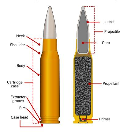
**Figure 2.14** Cross-sectional diagram showing key components of a contemporary (rimless, centrefire) rifle cartridge, in this case a 7.62 × 51 mm cartridge (source: ARES).
