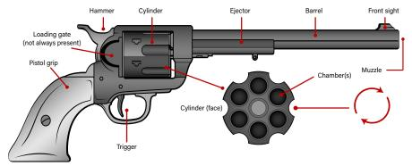
Figure 2.9 Typical parts of a revolver, in this case a single-action model (sources: ARES).
