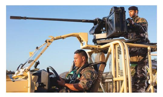
**Figure 2.47** A Nexter P20 (20 × 102 mm) light cannon, mounted on a military vehicle. In recent years, light cannon such as this have been positioned as replacement armaments for .50-calibre machine guns on light tactical vehicles (source: Nexter).
