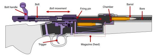
Figure 2.39 A cutaway diagram of a typical bolt-action rifle (source: ARES).
