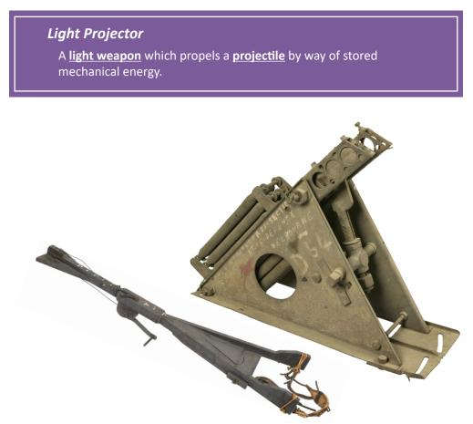
**Figure 2.61** Two light projectors. left: a Leach–Gamage Catapult, which used elastic rubber tubing to store mechanical energy. Right: a West Spring Gun, which employed several coiled springs to achieve a similar effect [not to scale] (sources: Imperial War Museum; Australian War Memorial).
