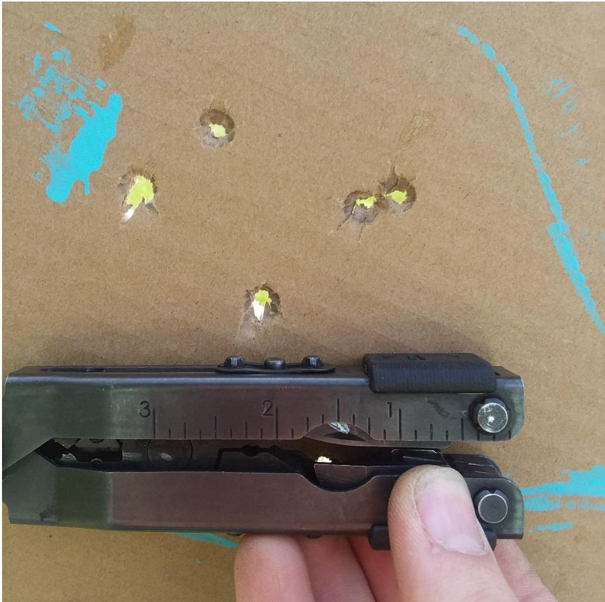
Figure 7.21 Informal testing of the precision achievable using an ECM-rifled 9 x 19 mm barrel (source: Ivan T./ARES).
