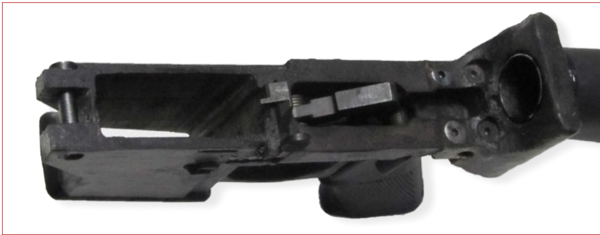
Figure 7.3 Commercially available FCG parts fitted to a 3D-printed AR-15 lower receiver (source: Ivan T./ARES).
