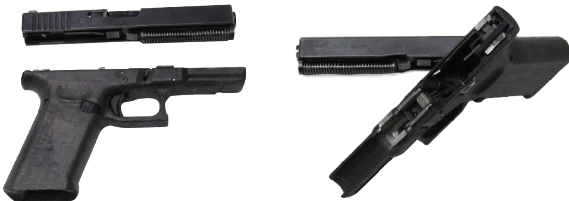
Figure 7.4 A Glock 17 frame printed in DuPont 'Zytel' glass-filled nylon. Factory Glock pistols use a near-identical polyamide 66 type material. Note the visible metal rails at right (source: Ivan T./ARES).
