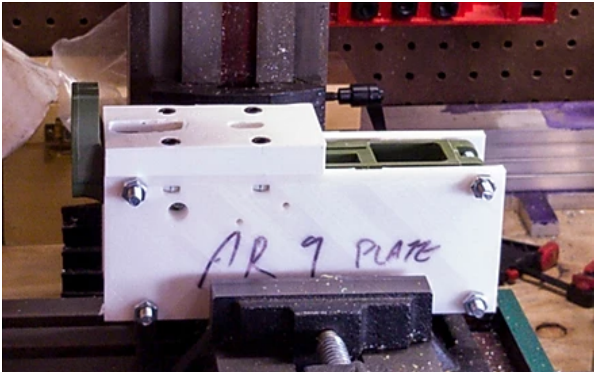
Figure 7.30 A 3D-printed receiver milling jig for AR-15-type '80% lowers' (source: Ctrl+Pew).
