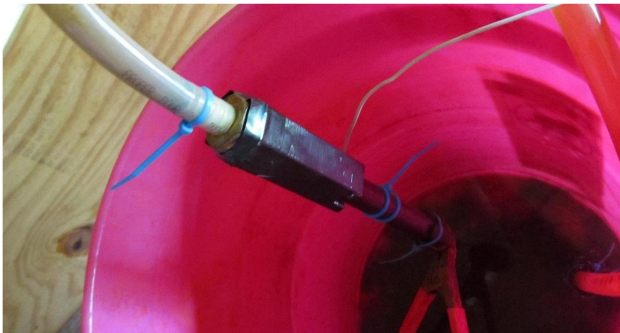
Figure 7.20 The ECM boring process in action (source: Ivan T./ARES).
