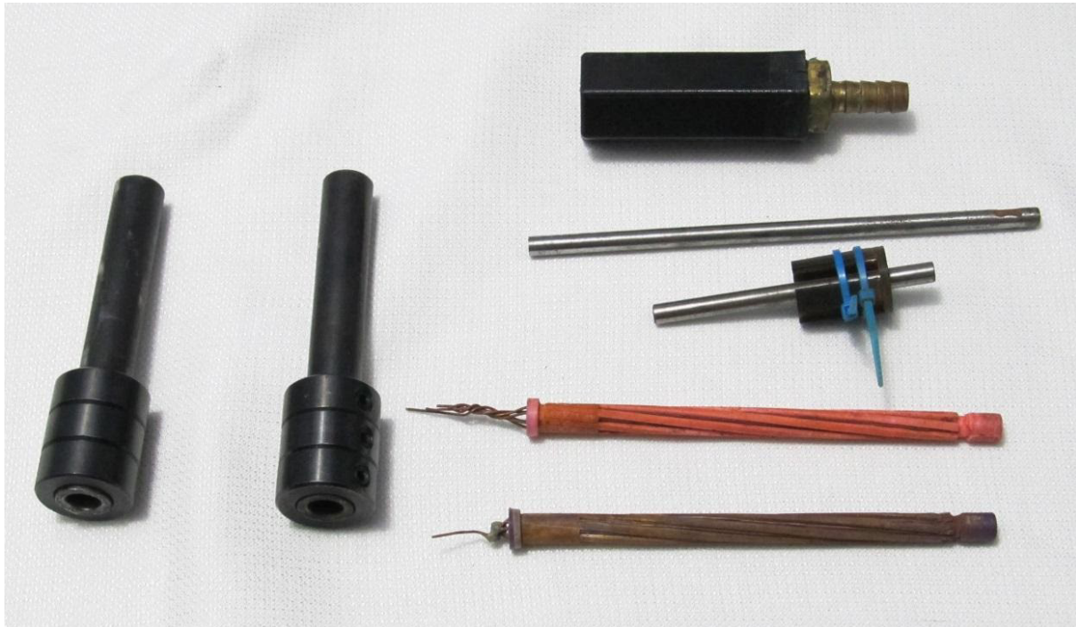
Figure 7.19 Two finished FGC-9 barrels (left) and the 3D-printed cathodes, jigs, and materials used (right) (source: Ivan T./ARES).
