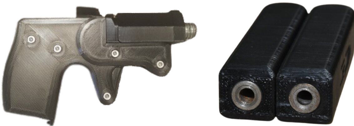
Figure 5.8 Left: A Harlot pistol with a threaded metal barrel protruding (source: Black Lotus Coalition). Right: Removable barrel units for PM422 Songbird 3D-printed single-shot pistols seized during an August 2020 raid in the western suburbs of Sydney, Australia. Note the reinforcing steel tubes sleeved into the printed barrel bodies (source: NSW Police Force).
