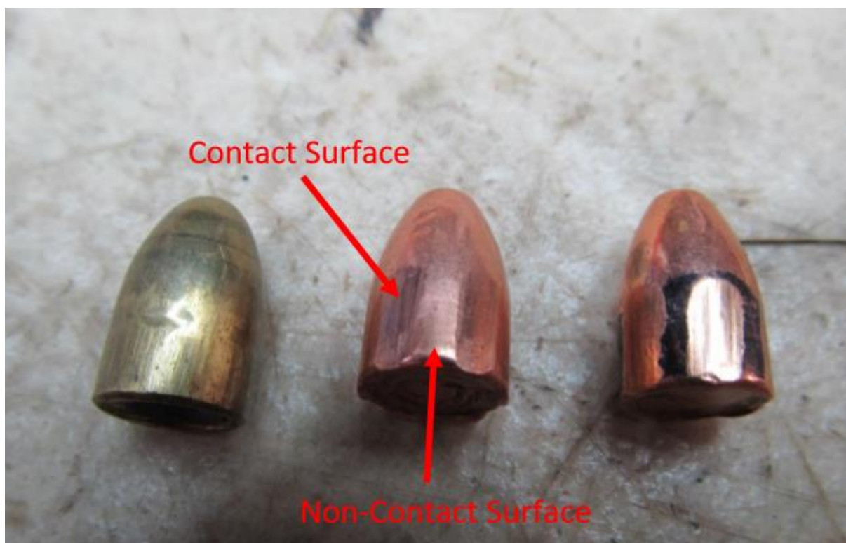
Figure 7.22 Above: the resulting rifling grooves produced inside the bore of the barrel are the inverse of those of the 3D-printed ECM guide. The horizontal striations are particularly characteristic of the 3D-printed mandrels used in this particular ECM process, which are printed upright. Below: Distinctive rifling marks on a ‘slugged’ bullet indicate a successfully produced barrel (source: Ivan T./ARES).
