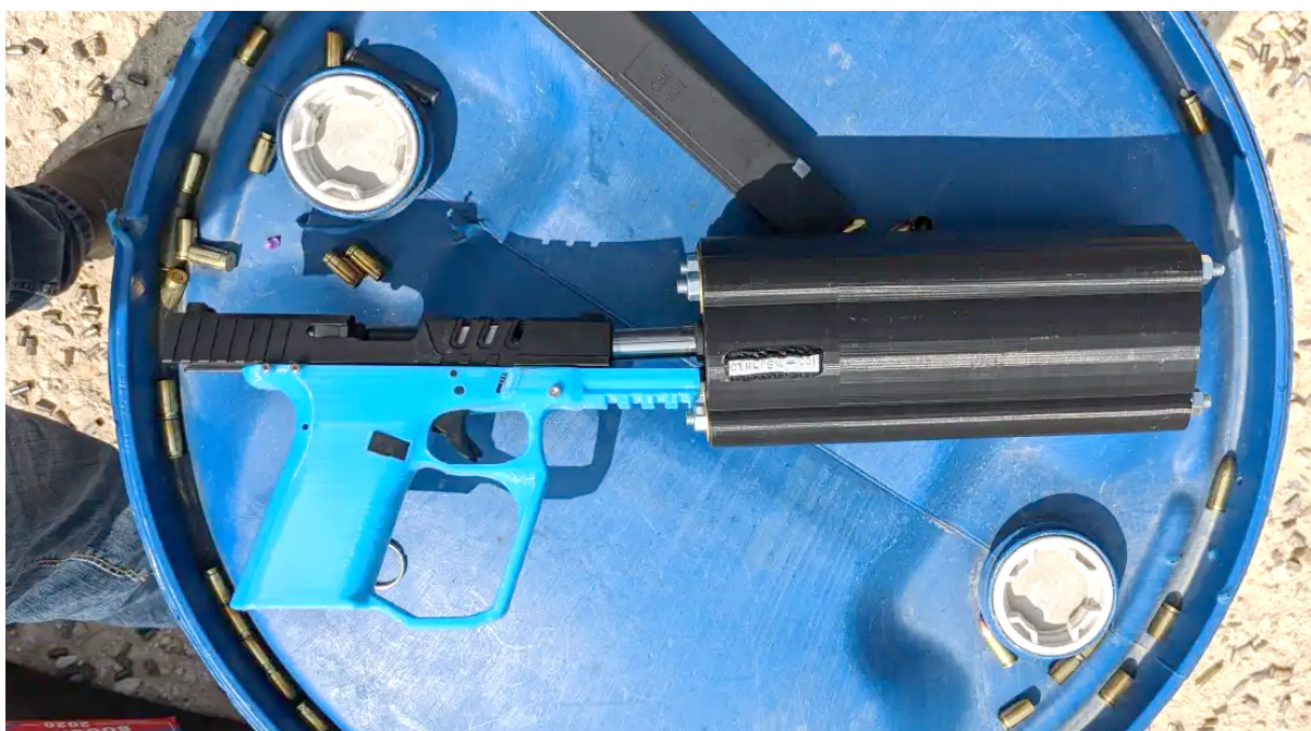
Figure 7.28 The 3D-printed ‘Shush Puppy’ suppressor. Note its bulky design, which allows it to fire more powerful cartridges (source: CTRL+Pew).
