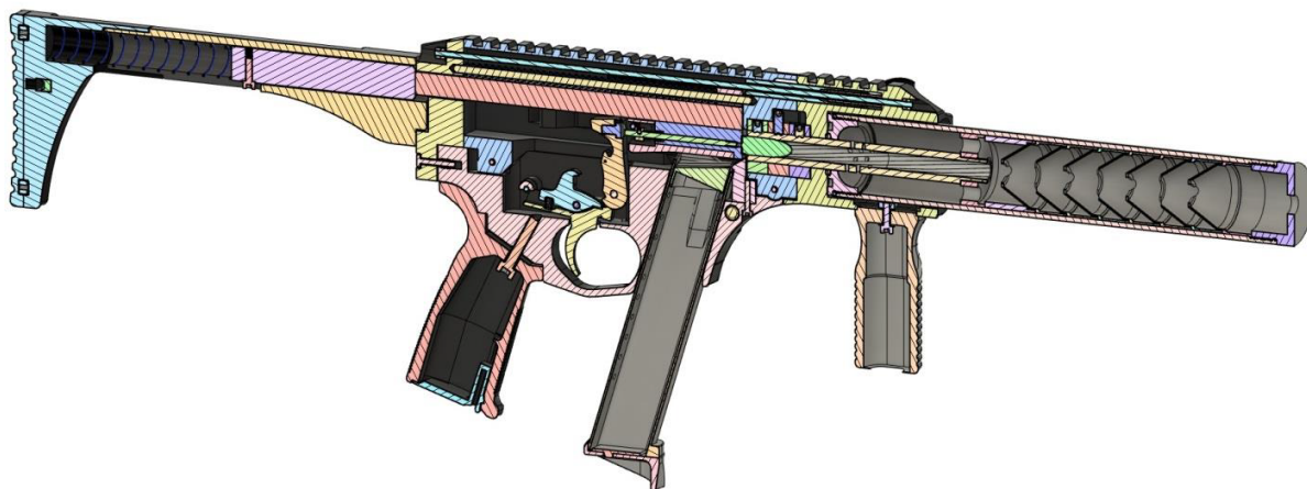
Figure 5.16 A rendering of a Partisan 9 equipped with a ported barrel and suppressor. Note the holes indicated roughly mid-way in the rifled barrel (source: The_Real_BrOletariat ).
