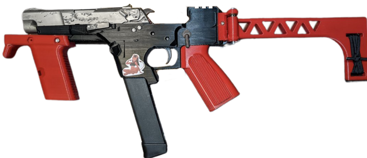
Figure 5.25 A Recession Ruger with a 3D-printed side-folding stock and a picatinny rail to mount an optic (source: DrDeath1776).
