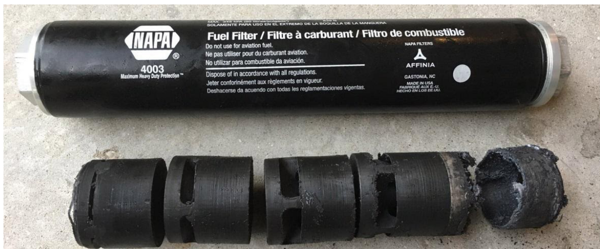
Figure 7.26 KadeCAD baffles and the fuel filter tube they reside into after reportedly being subjected to 150 rounds of continuous fire using .223 Remington ammunition (source: KadeCAD on Twitter; Hays, Ivan T., & Jenzen-Jones, 2020).
