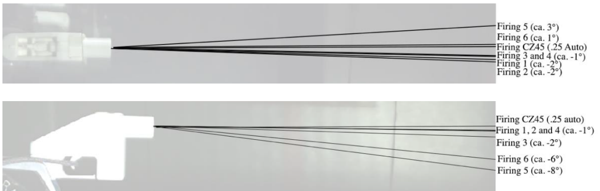
Figure 5.7 Vertical and Lateral trajectories of the six projectiles fired from six Liberators with a shot from an industrially made CZ45 as comparison (source: Honsberger, et al.).
