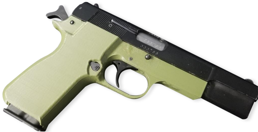
Figure 7.9 A Browning Hi-Power self-loading pistol with a 3D-printed frame (source: Ivan T./ARES).
