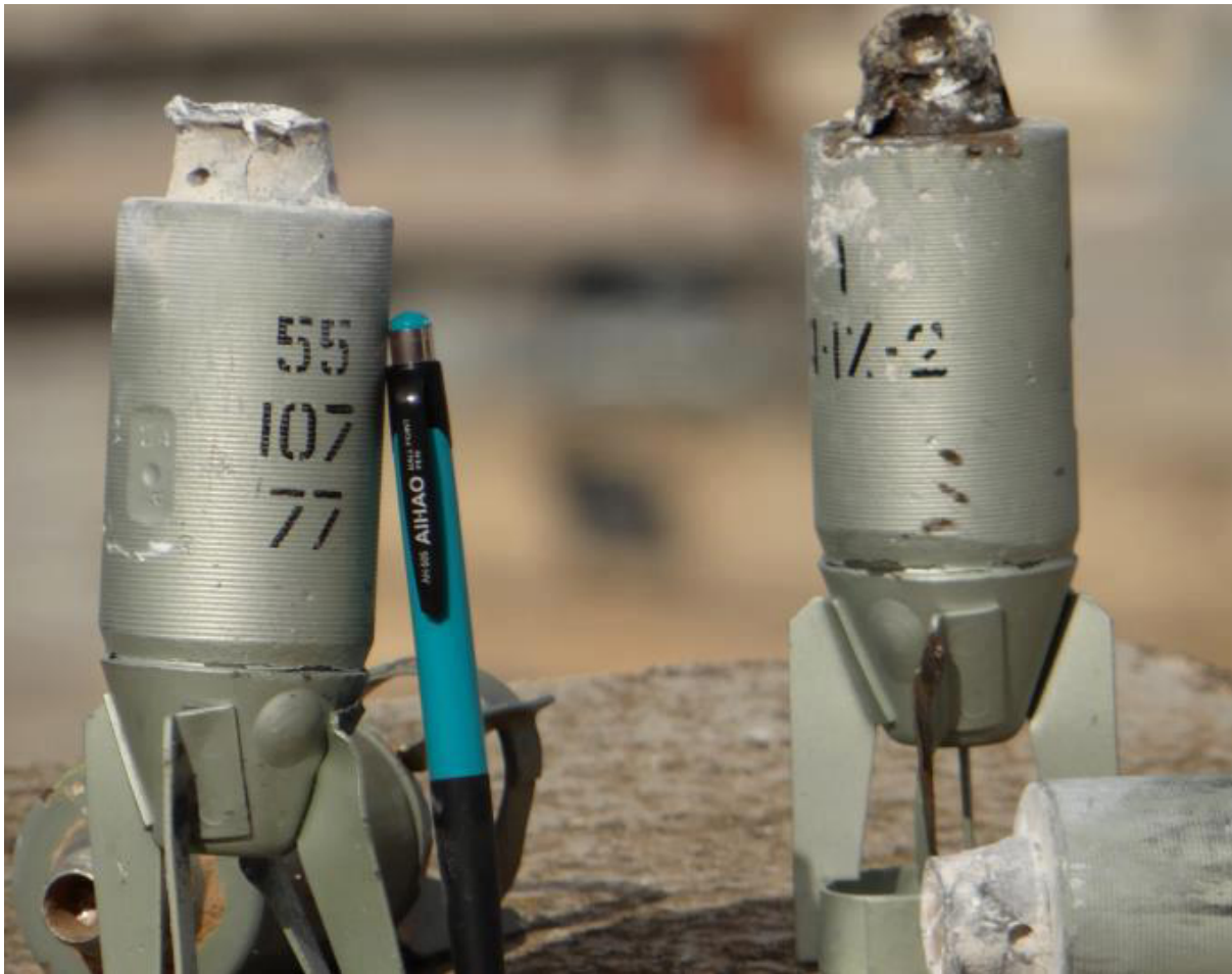
Figure 2.2 Unexploded AO-1Sch submunitions identified in Maarrat al-Numan, Idlib, with a pen for scale. The markings on the left-hand submunition indicate factory number, lot number, and year of production. Markings on the right-hand submunition read “A-IX-2”, designating the explosive fill (source: Syrian social media via ARES CONMAT Database).
