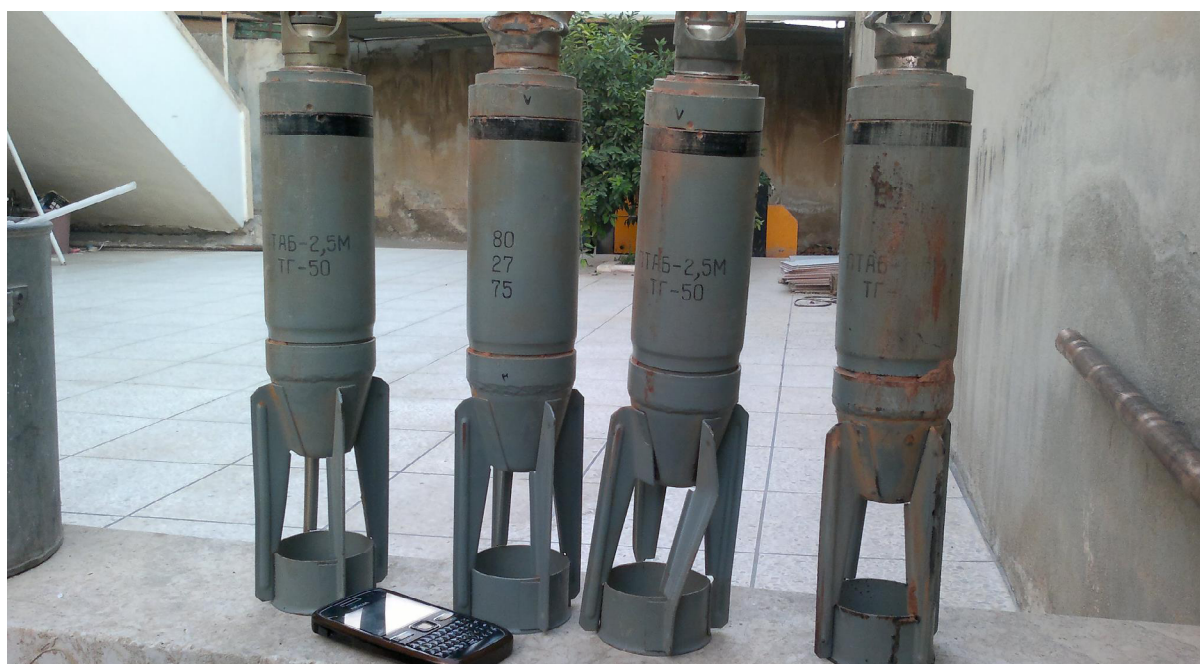
Figure 2.35 PTAB-2.5M submunitions recovered in Syria. Translated, the markings on these munitions read “PTAB-2.5M” and, below, “TG-50” (the explosive fill). The reverse side, as seen on the submunition second from the left, displays factory code (80), lot number (27), and year of production (1975) (source: Syrian social media via ARES CONMAT Database).
