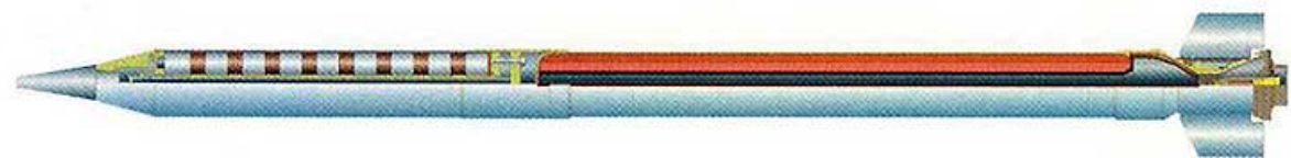
Figure 1.6 9M218 cargo rocket with anti-tank submunitions. Representative of the general layout of 122mm cargo rockets (source: missilery.info ).
