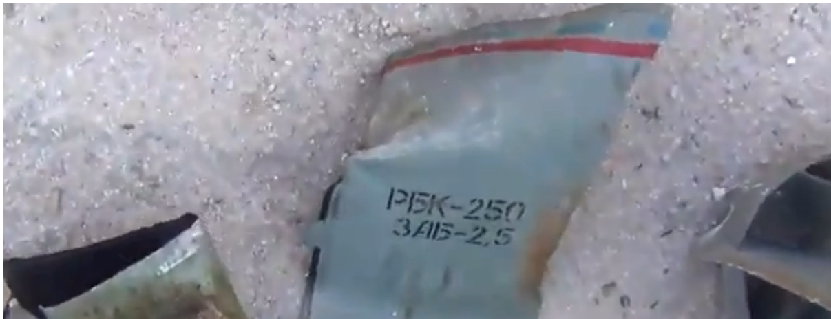
Figure 2.67 The remains of a bomb found in the Aleppo Governorate in November 2012. The markings indicate this is an RBK-250 ZAB-2.5 (source: Syrian social media via ARES CONMAT Database).
