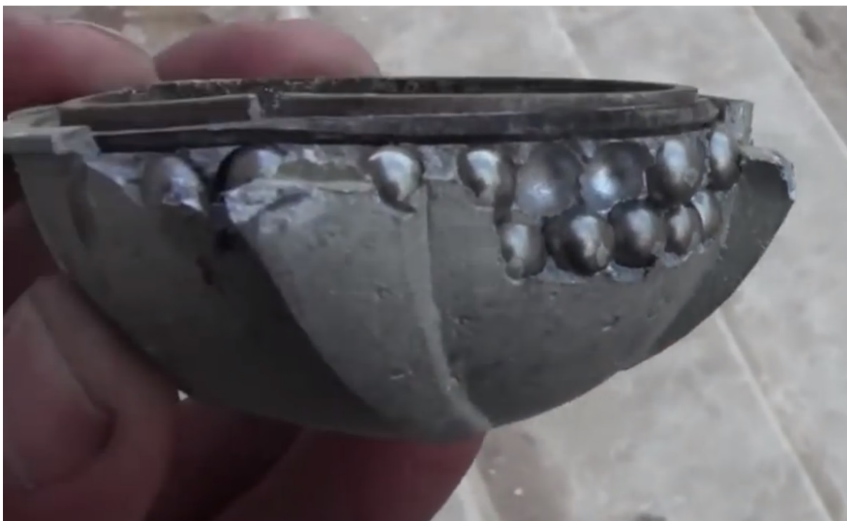
Figure 2.21 A Syrian displays remnants from the body of a ShOAB-0.5 submunition in March 2013, with steel balls used as fragmentation visible (source: Syrian social media via ARES CONMAT Database).
