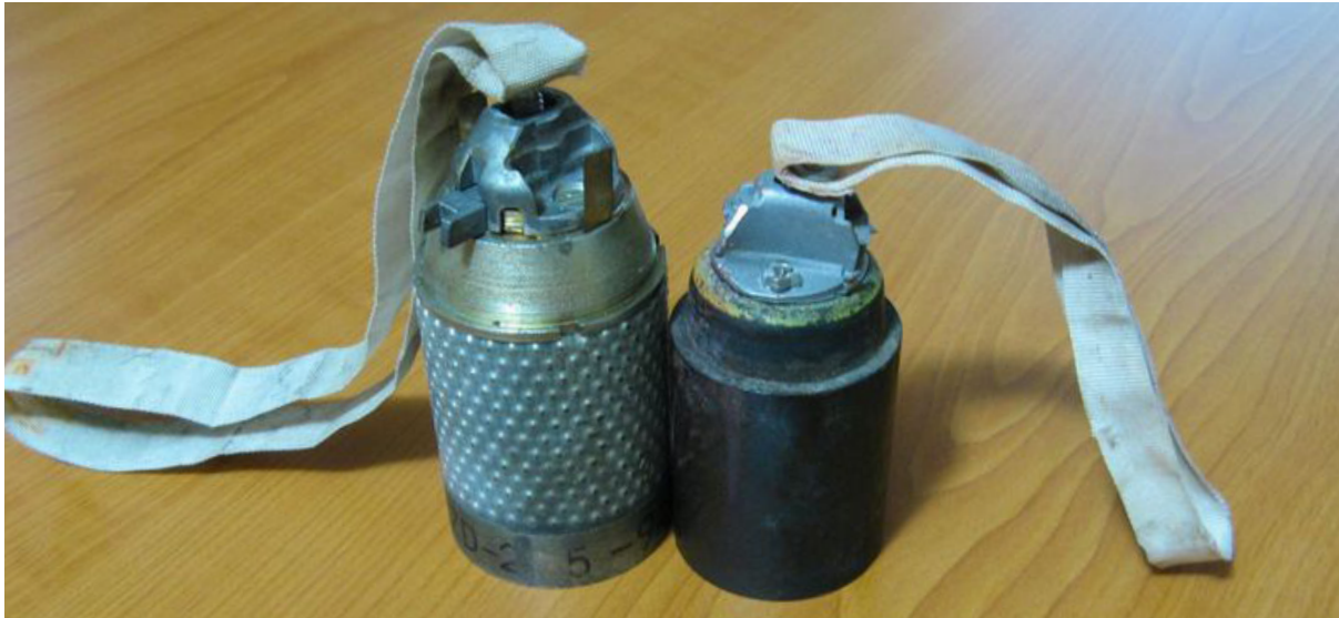
Figure 2.55 Size comparison between an MZD-2 (left) and a Sakr Type B (right). Note the spherical pre-formed fragmentation visible in the clear polymer matrix of the MZD-2, as well as its larger, distinctive shape (source: Mizokami, 2016).
