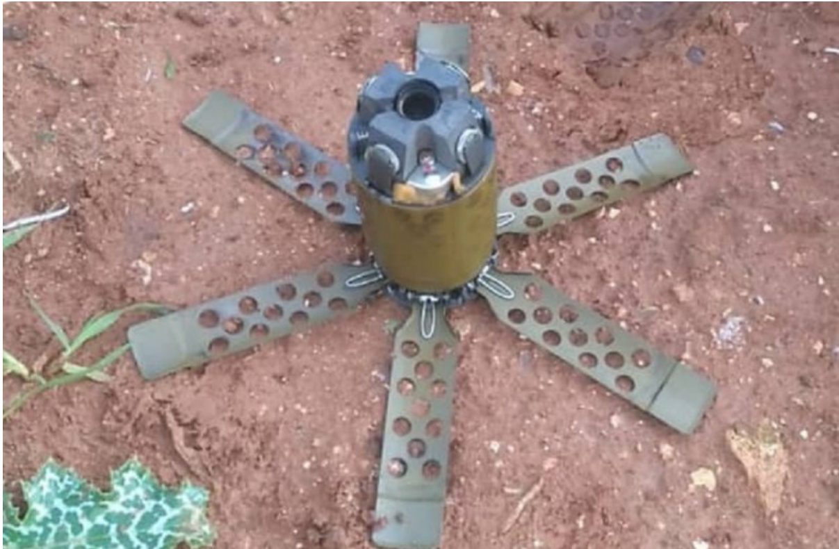
Figure 3.8 A POM-2 mine that failed to deploy its tripwires, pictured in northern Syria in January 2019 (source: Syrian social media via ARES CONMAT Database).
