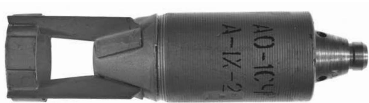
Figure 2.1 An AO-1SCh submunition (source: Russian Social Media via ARES CONMAT Database).
