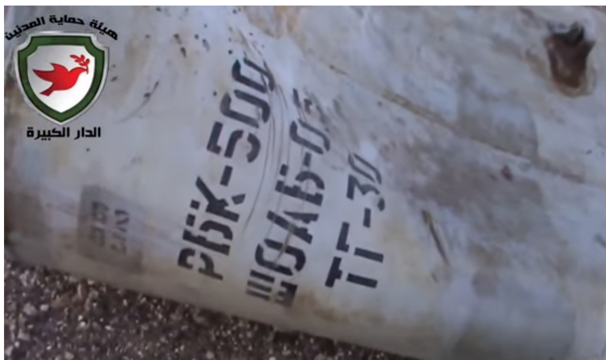
Figure 2.22 The remains of a cluster bomb in Homs, Homs Governorate, in April 2013. The markings on the side are translated as “RBK-500 ShOAB-0.5” and underneath “TG-30”, indicating the explosive compound within the submunitions (source: Syrian social media via ARES CONMAT Database).
