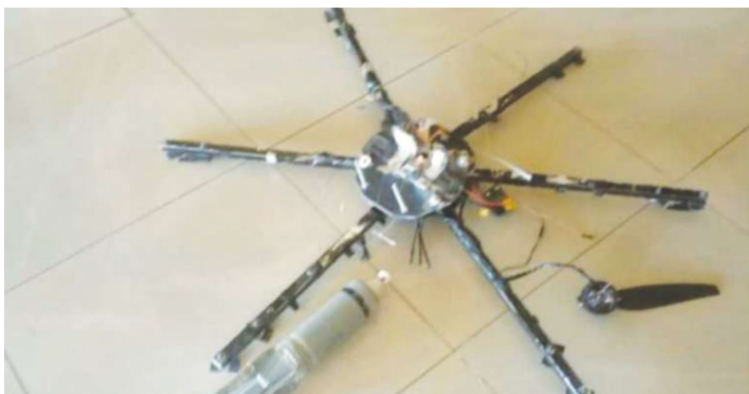
Figure 3.17 An intercepted commercial UAV with a modified PTAB-2.5M munition (source: Syrian social media via ARES CONMAT Database).
