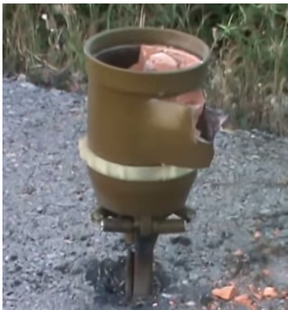
Figure 3.3 Another Type 84 mine near Sawaysa. Like in Figure 3.2, this mine appears to have been shot in an effort to disable it, with the body of the mine broken and explosive composition spilled out (source: Syrian social media via ARES CONMAT Database).
