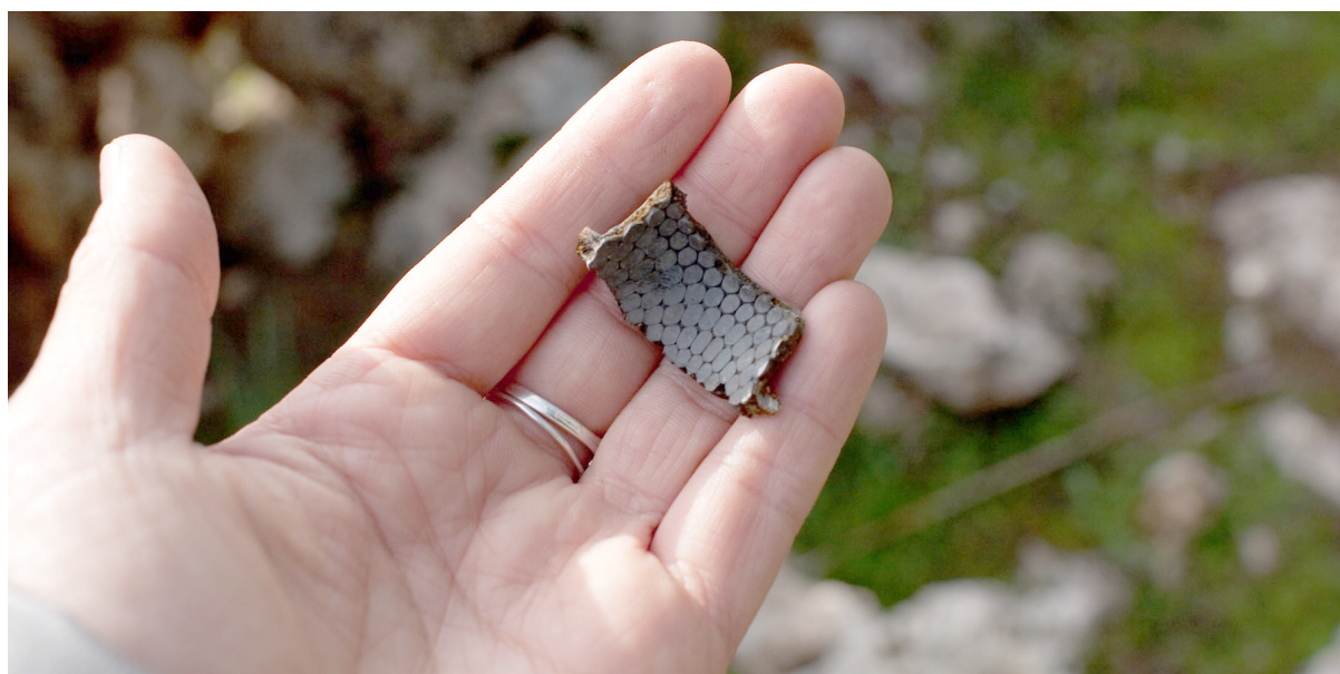
Figure 2.47 A piece of Sakr Type B submunition body showing its fragmentation sleeve. Jabal al-Zaweya, December 2012 (source: Nicole Tung).
