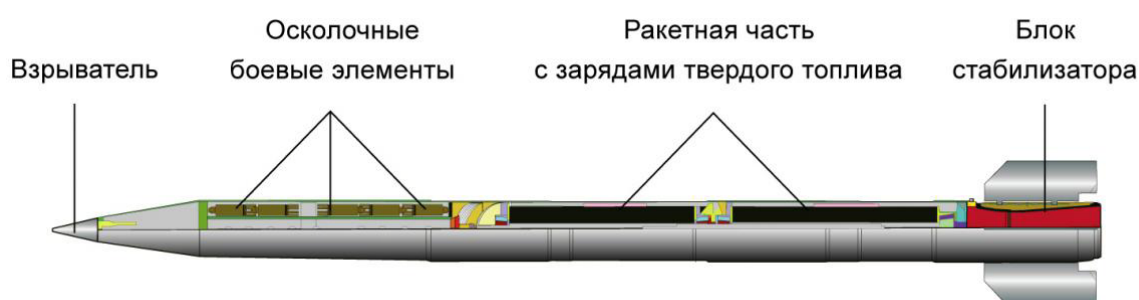
Figure 1.8 9M27K cargo rocket with 9N210 fragmentation submunitions (source: missilery.info ).
