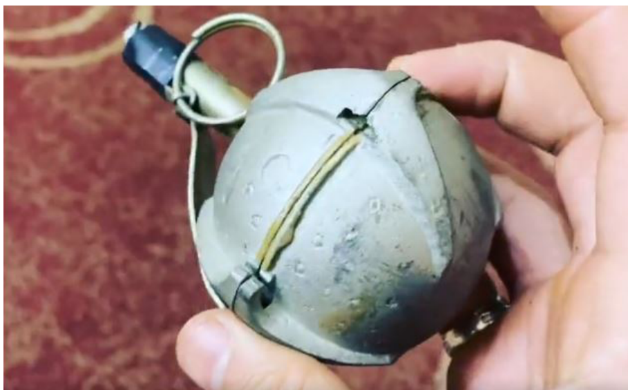
Figure 3.13 A repurposed ShOAB-0.5 HE-FRAG submunition fitted with a UZRGM-pattern fuze, creating an improvised hand grenade (source: Syrian social media via ARES CONMAT Database).
