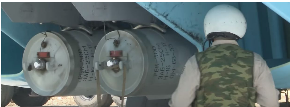
Figure 2.71 RBK-500 ZAB-2.5SM aerial bombs mounted under the wings of a plane stationed at the Russian Khmeimim airbase in Syria. Taken from a Russia Today report which aired on 18 June 2016. Note the markings on this RBK-500 ZAB-2.5SM indicating its contents: H-16 referring to the ZAB-2.5M1 containing N-16, H-17 referring to the ZAB-2.5M2 containing N-17, and OM-68-35 referring to the ZAB-2.5S containing OM-68-35 (source: RT).
