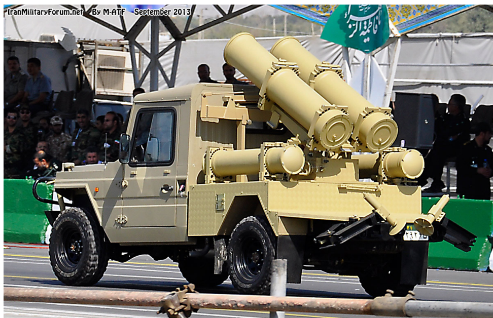
Photo 4 Sepehr tactical vehicle with FL1-A and FL2-A launch tubes on parade in Tehran.
